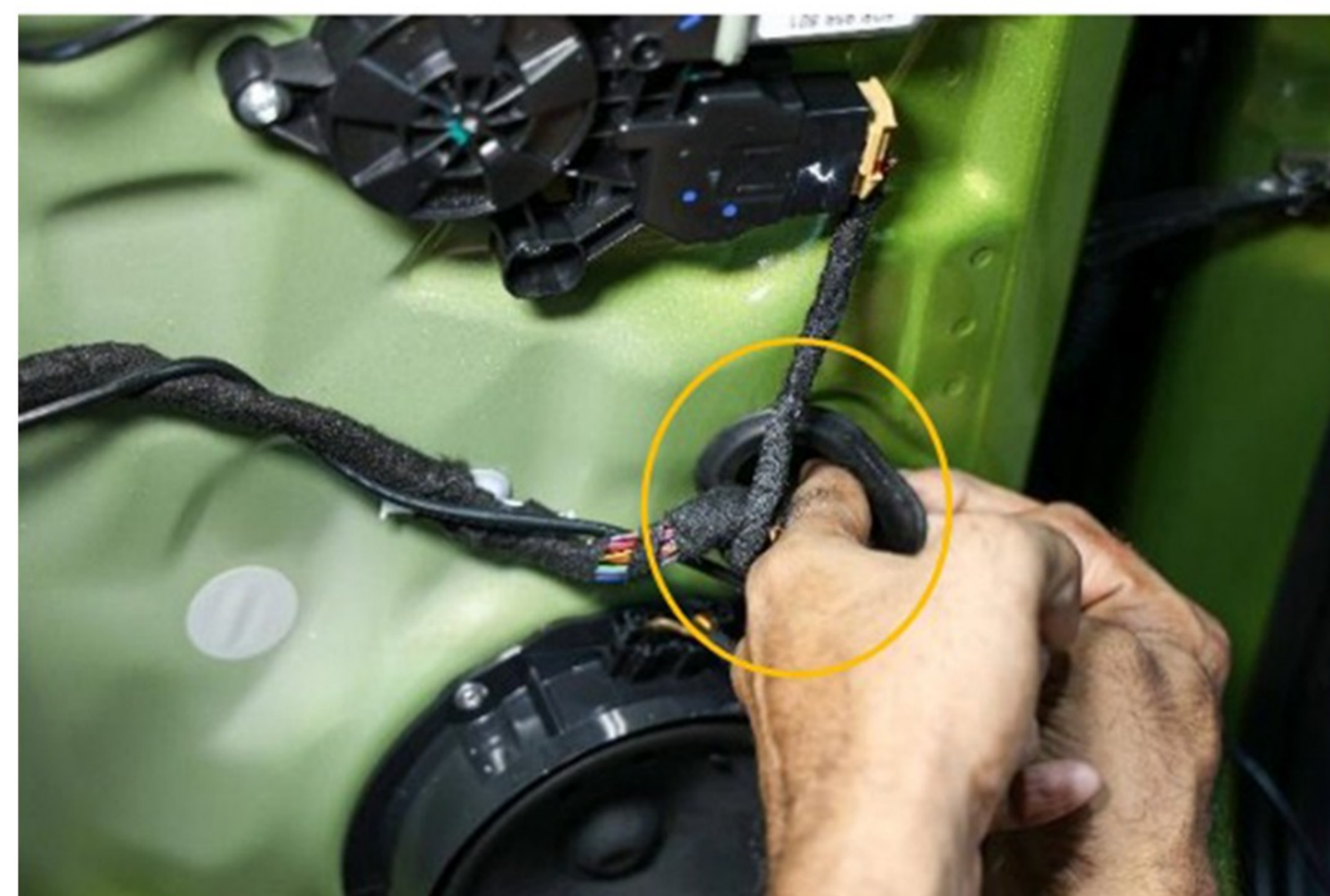
Step 46:- Route extension cable through the rubber grommet as shown in step 45
