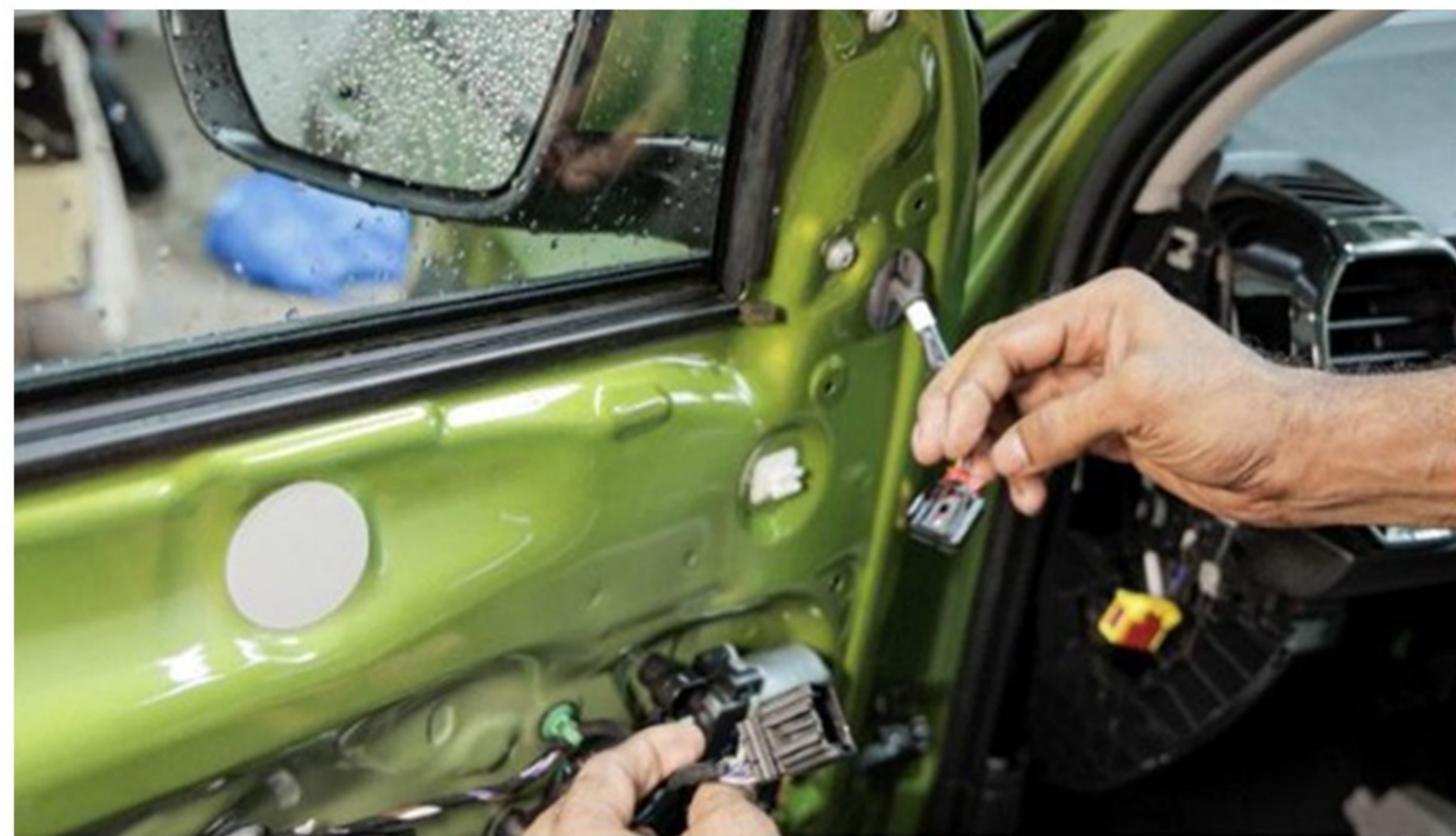
Step 29 :- Disconnect the ORVM Connectors
