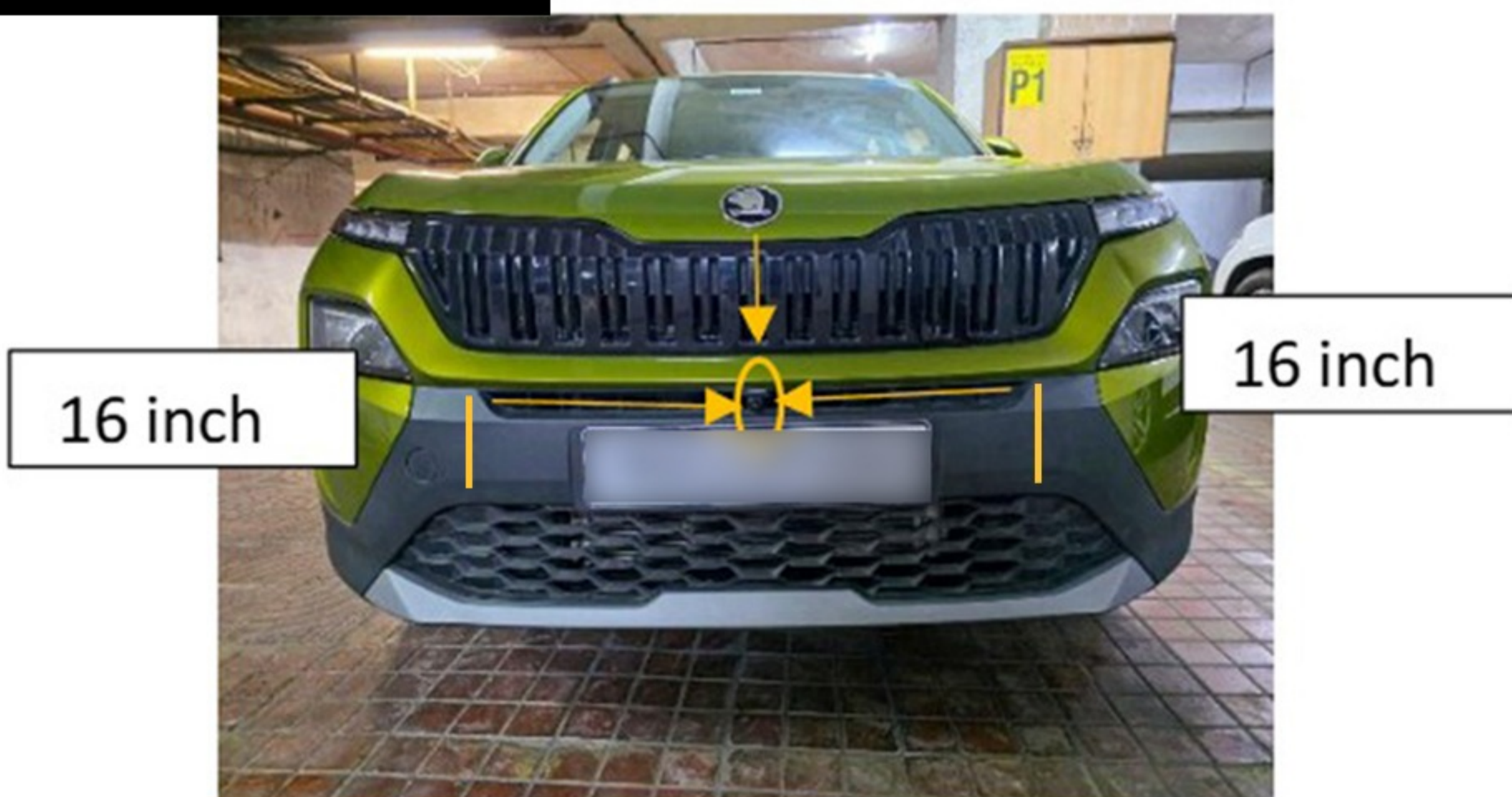
Step 79 :- Measure Length from Left and Right side as shown and place and Front Camera
