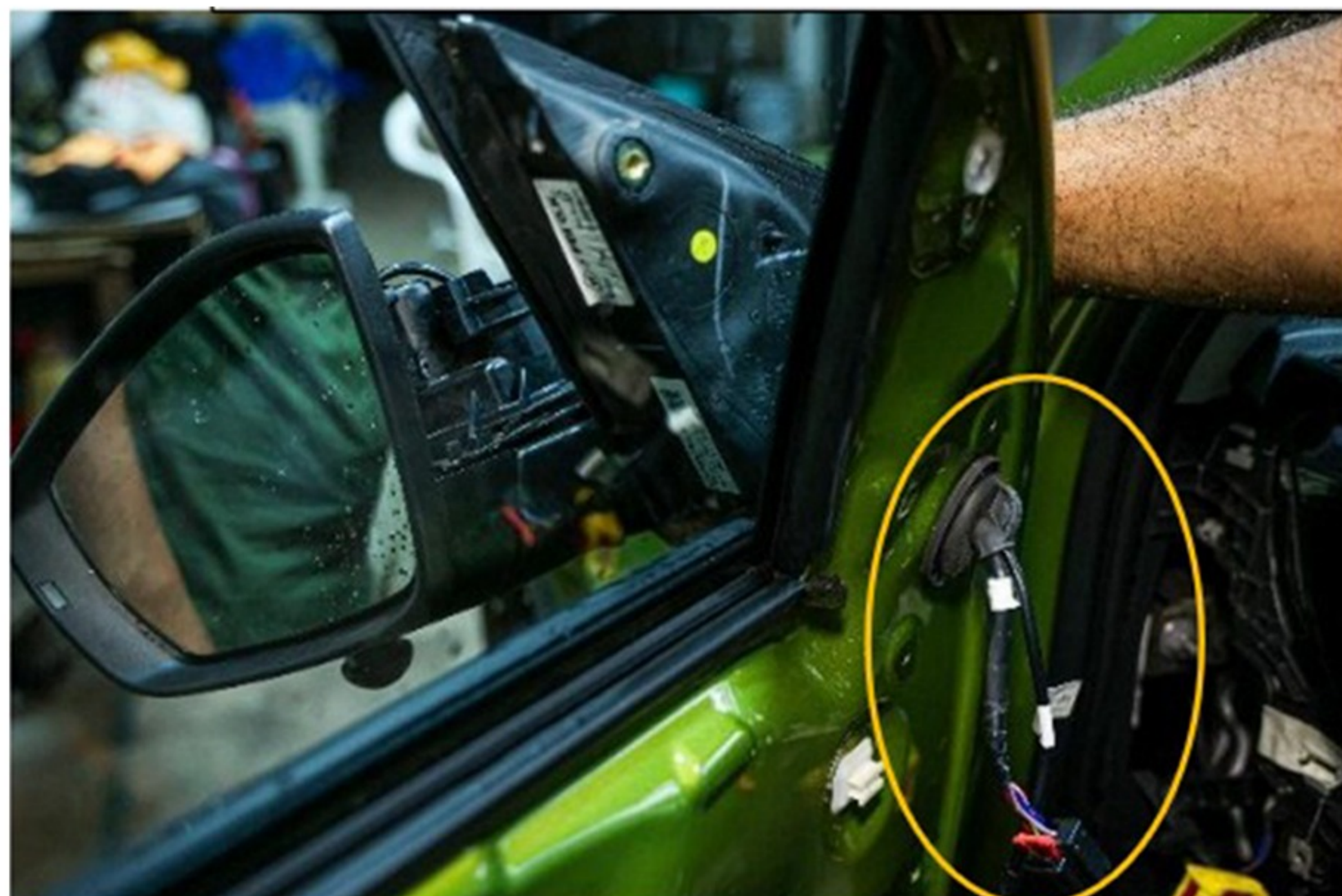
Step 39 :- Connect Left and Right ORVMS and route cables as shown
