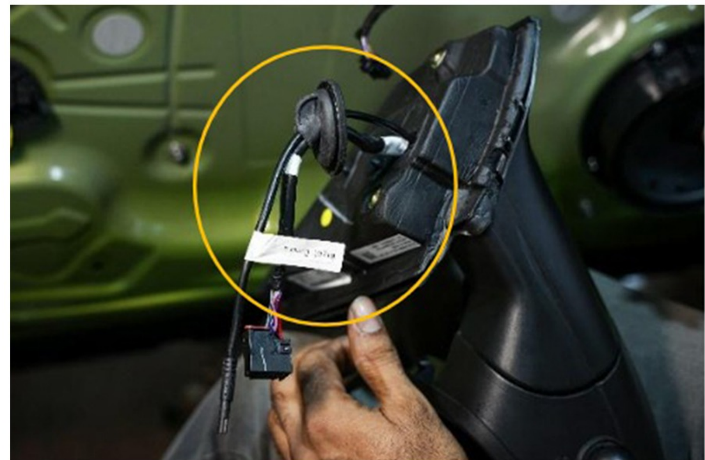
Step 38 :- Route cables as shown from rubber Grommet
