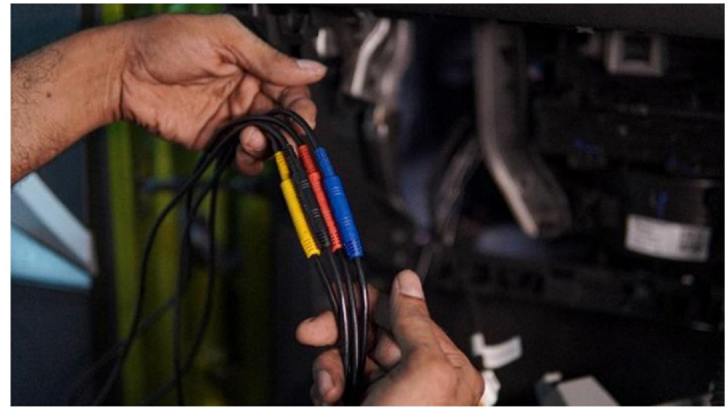
Step 91 :- Connect all 4 camera extension cables ( Part no 2,3,4,5) to the 32Pin power cord ( Part no 6) as shown
