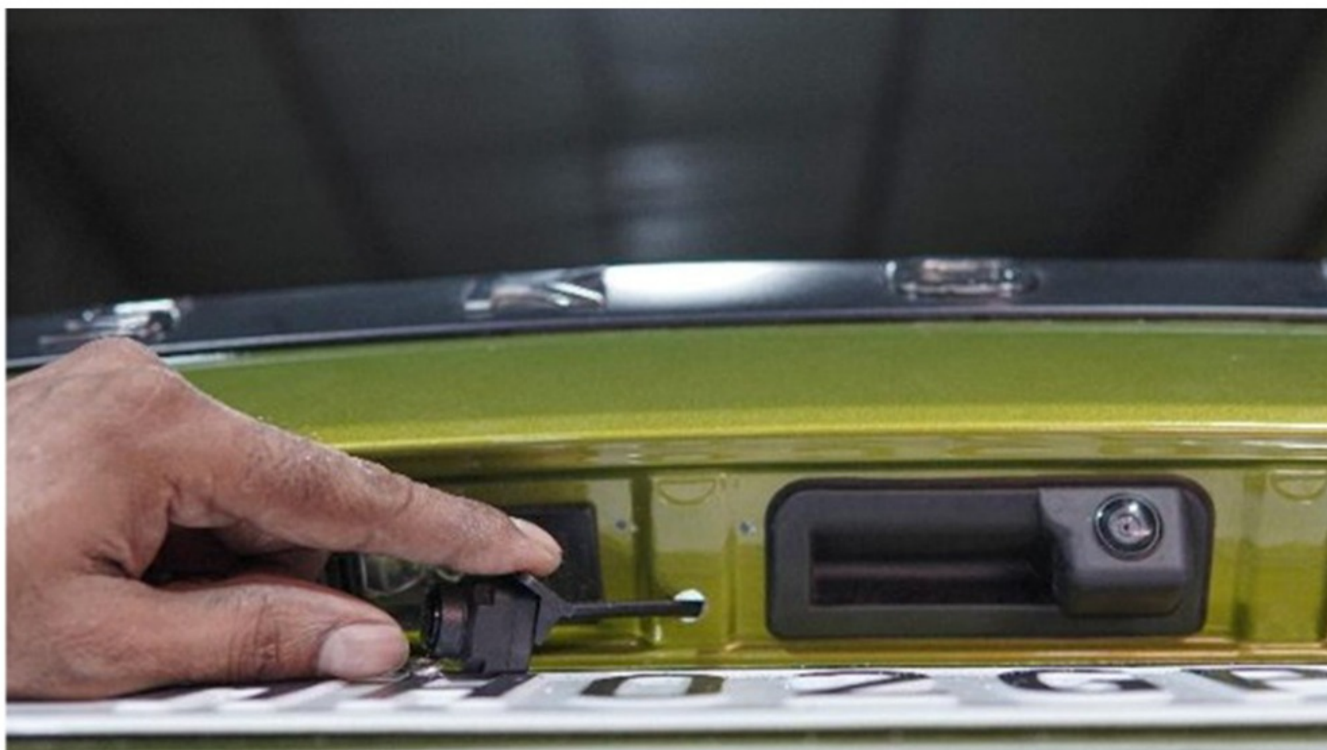
Step 99 :- Route rear camera (Part no 7) cable through the hole paint touch up to be done to avoid rusting if required
