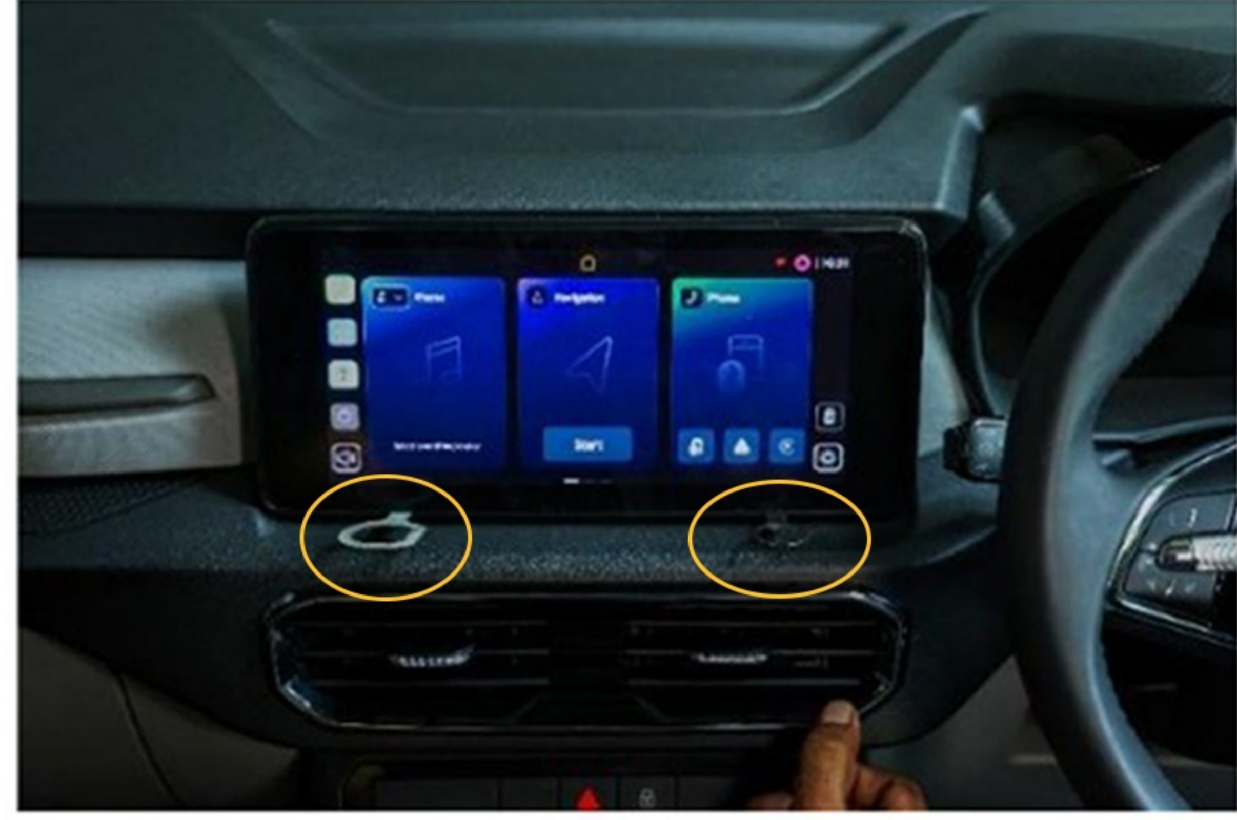
Step 2:- Insert PIN and disconnect Multimedia lock
