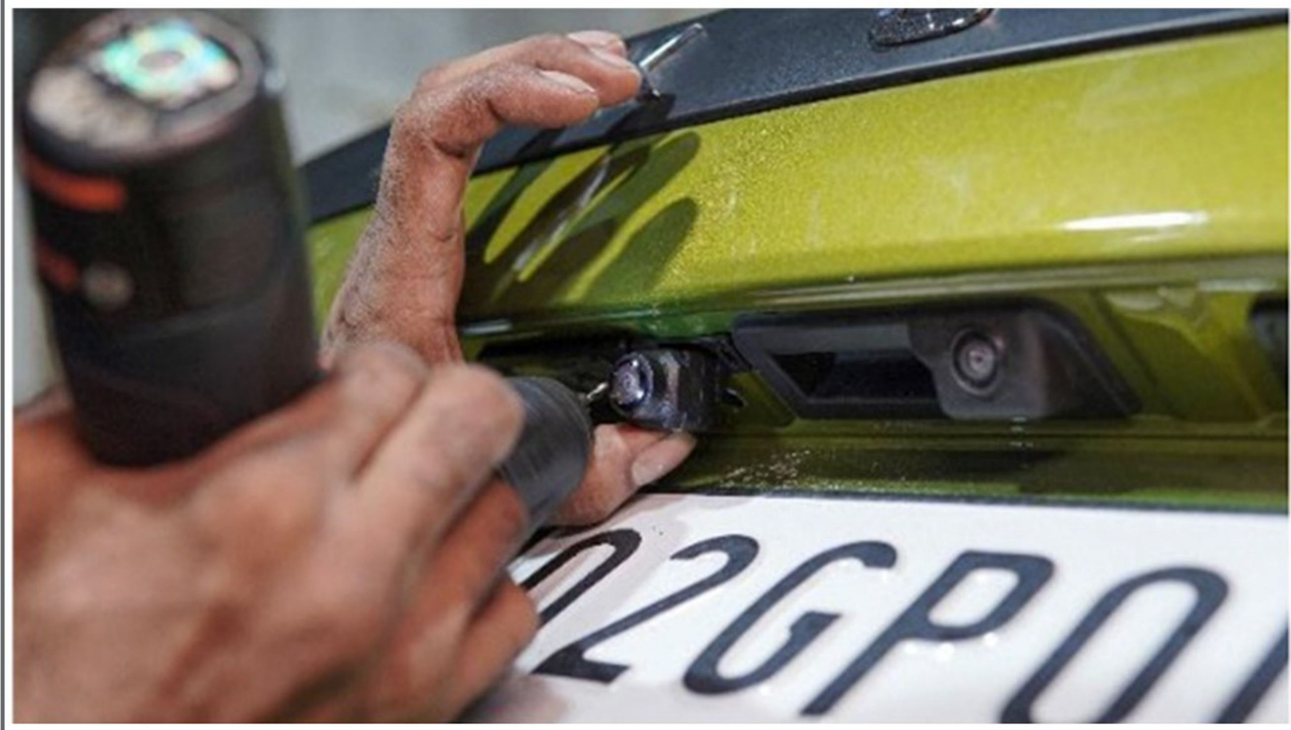
Step 100 :- Drill 2 small hole with the smaller holesaw ( Part no 17)2mm to fix the 2 screws (Part no 12) for rear camera
