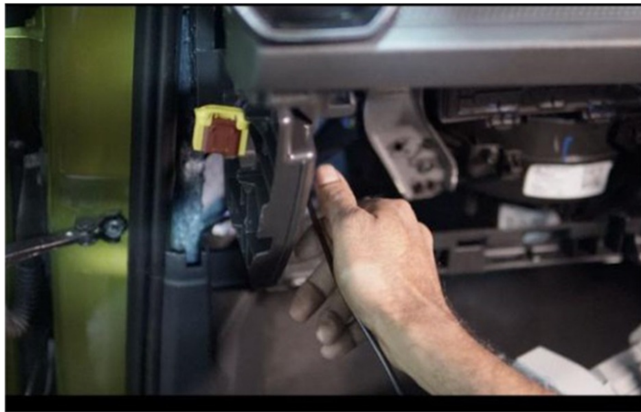
Step 90 :- Route cable through the rubber sleeve and to the glovebox area ( kindly refer the video if any confusion)
