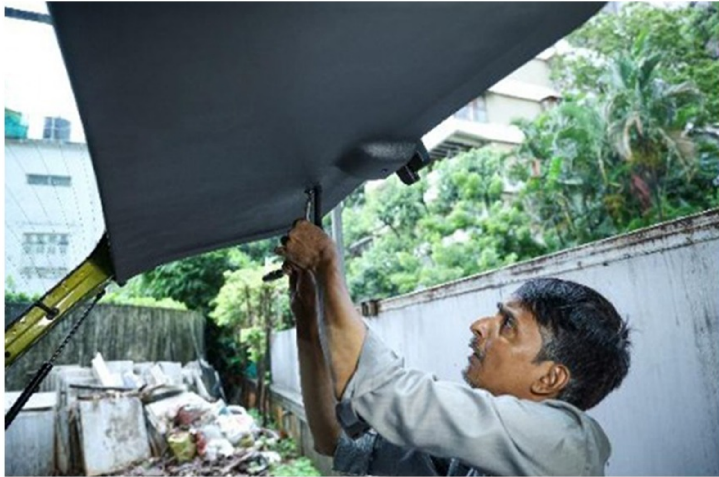
Step 59 :- Remove the tailgate Plastic Trim as per Series process.
