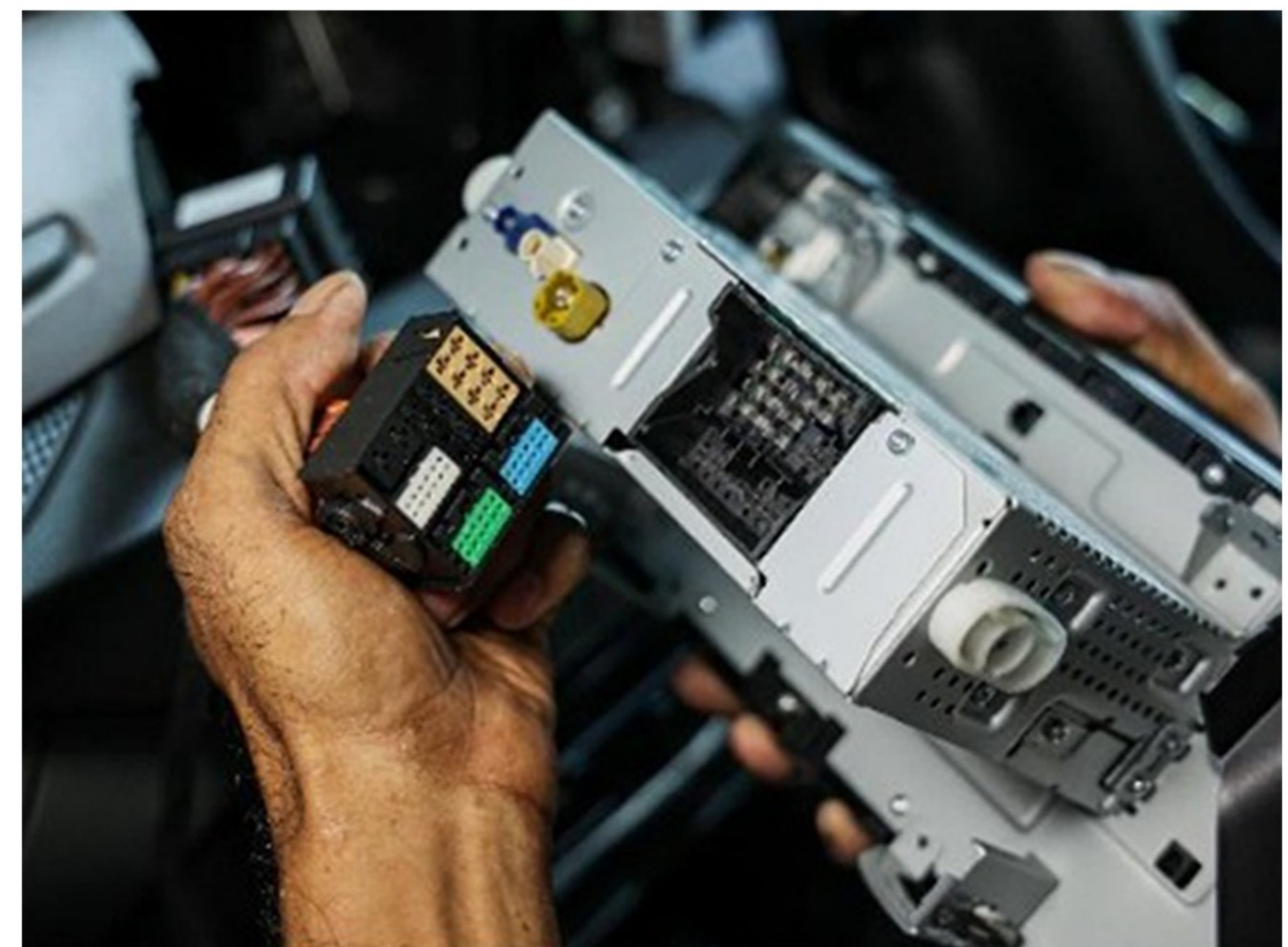
Step 8 :- Connect the other end of part (9) to series multimedia as shown on the sticker
