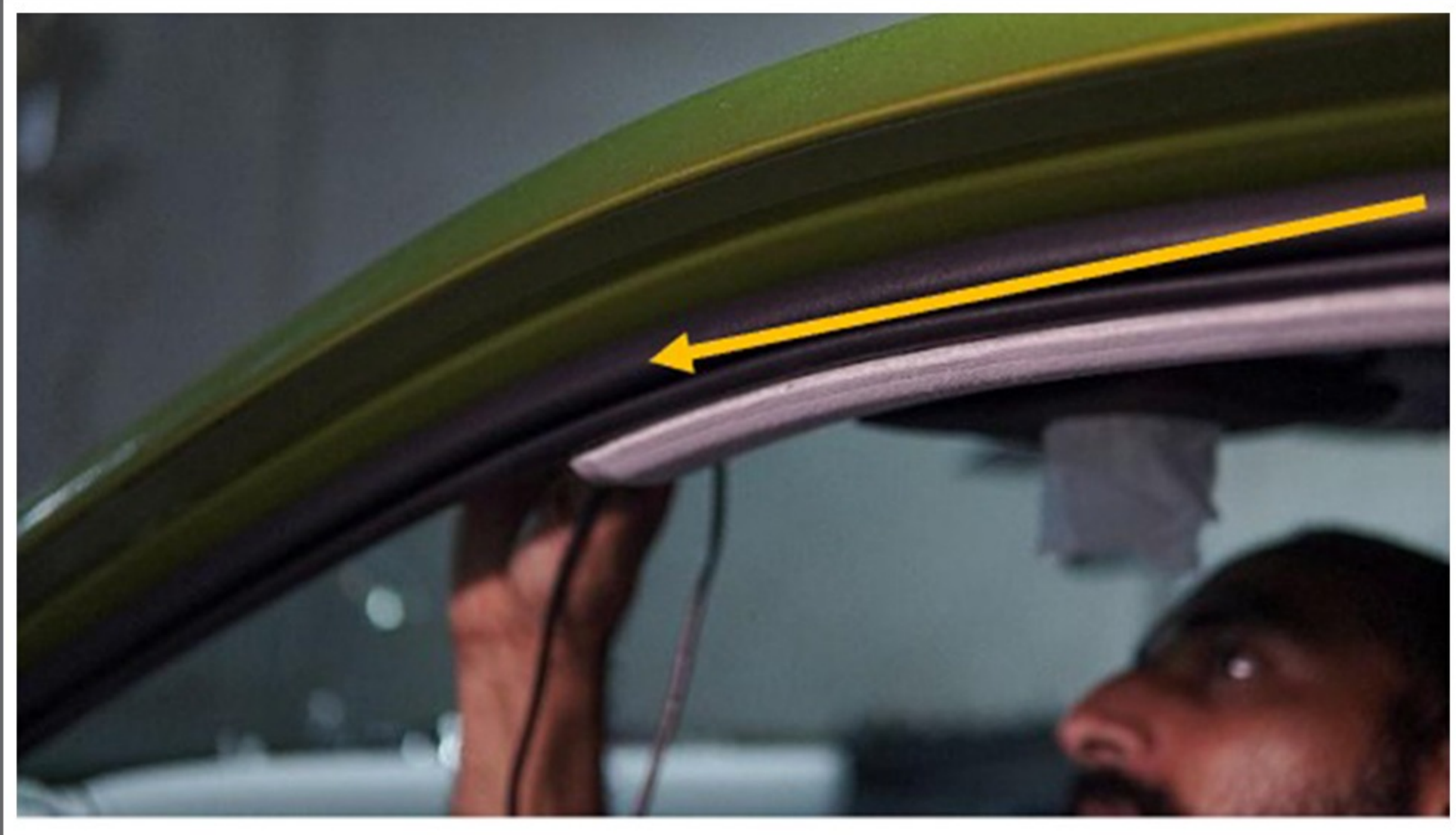
Step 74 :- Route cable through the Roof liner
