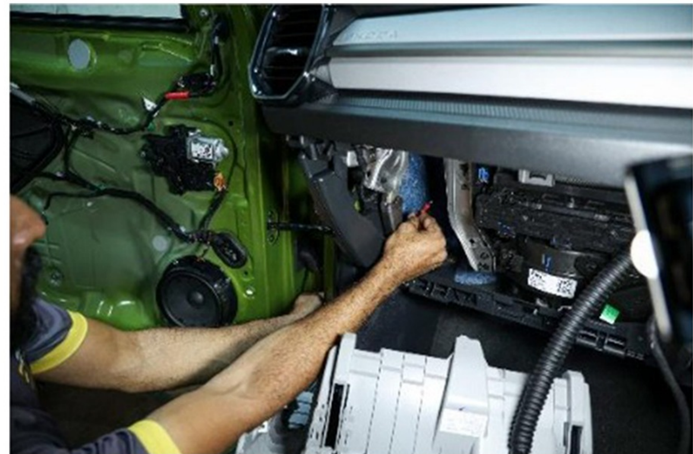
Step 50 :- After route through the hole, pull all the excess cable
