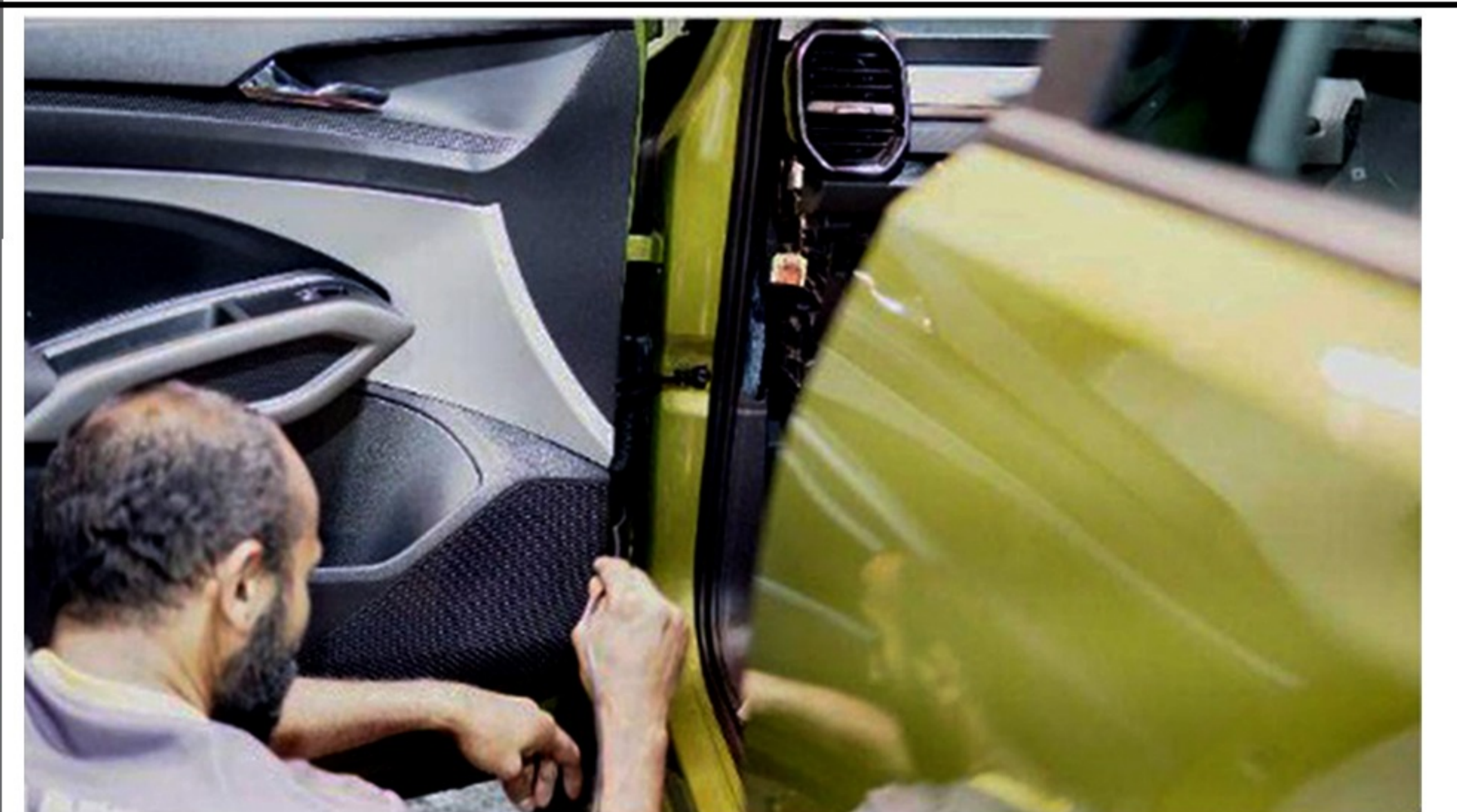
Step 89 :- Route cables as marked till glove box ( kindly refer the video if any confusion)
