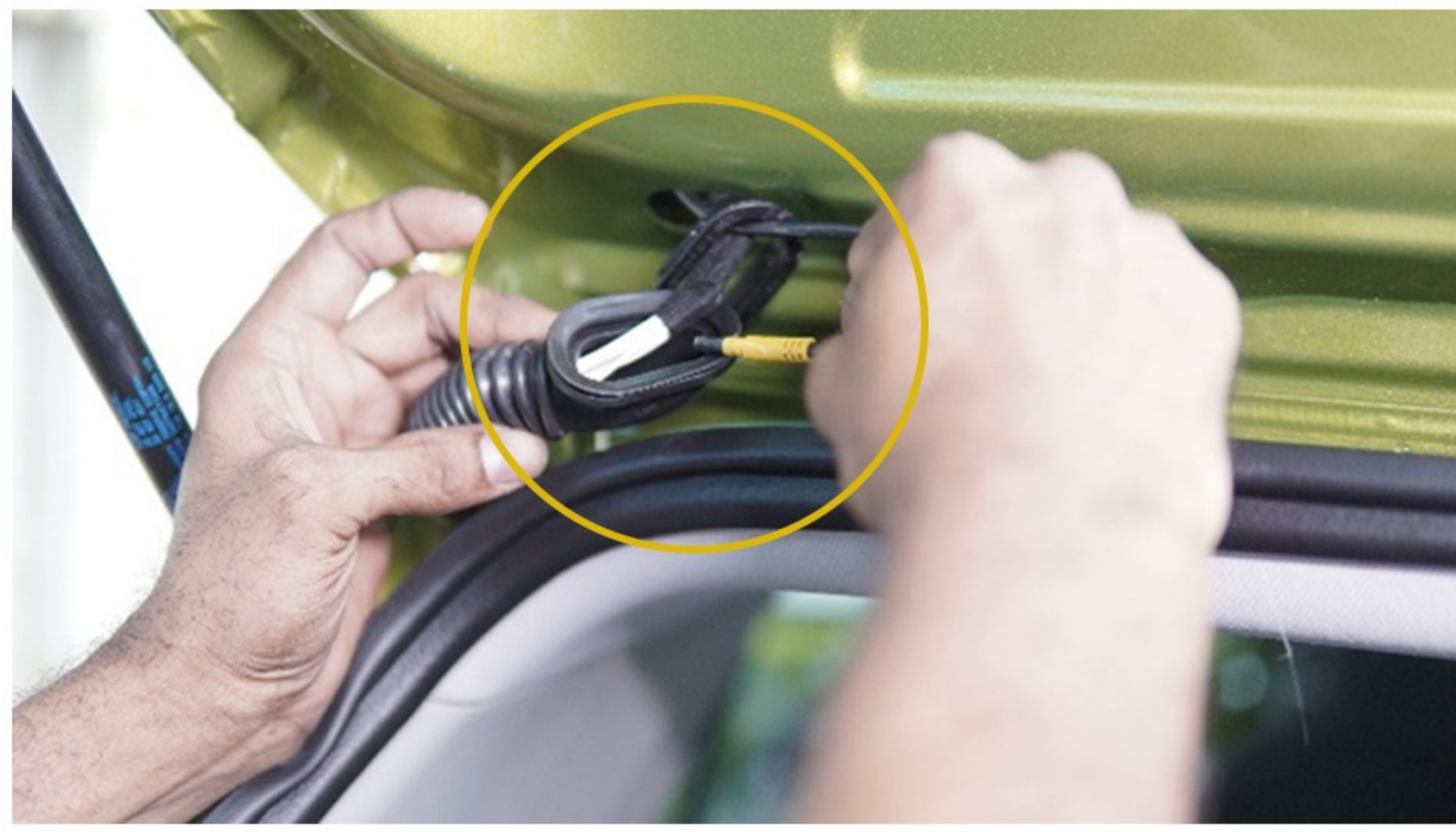
Step 65 :- Route Cable through the rubber sleeve
