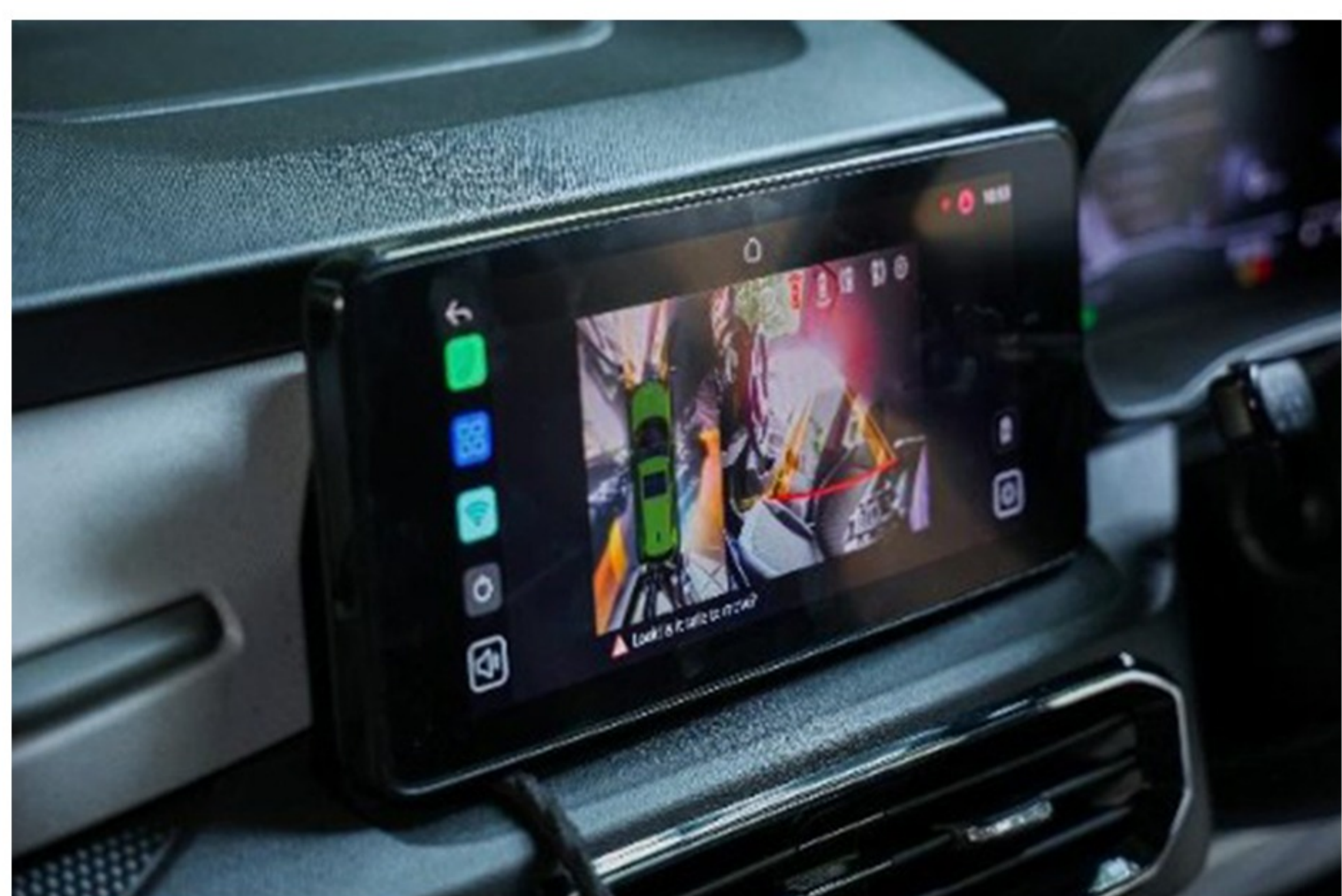
Step 16 :- Function Check all camera by the powering on Infotainment
