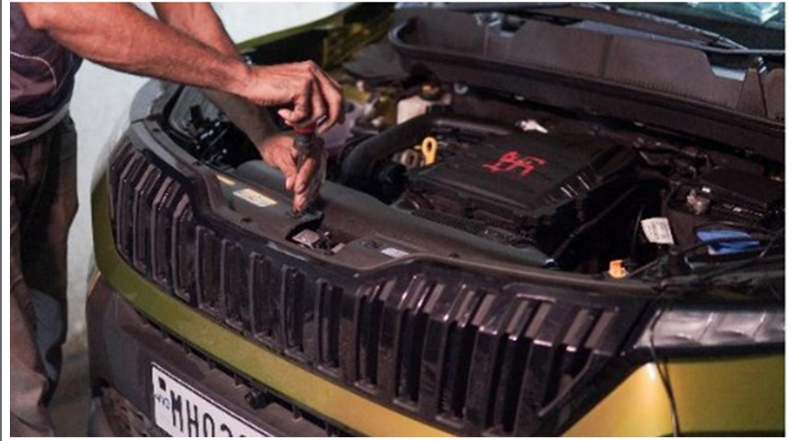
Step 83 :- Remove the bumper insert cover near engine bay as per series process
