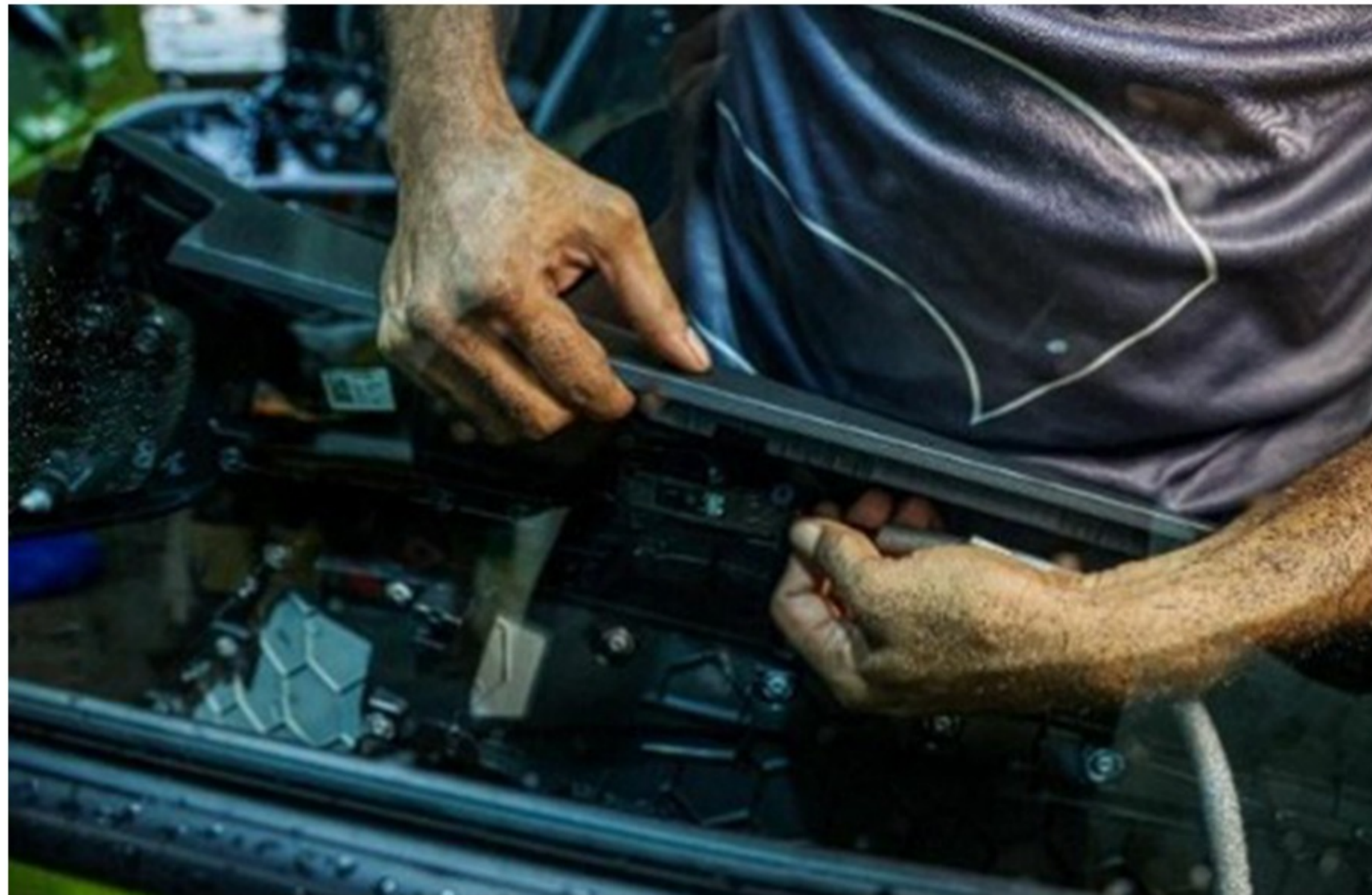
Step 27 :- Disconnect all connectors on the door panel
