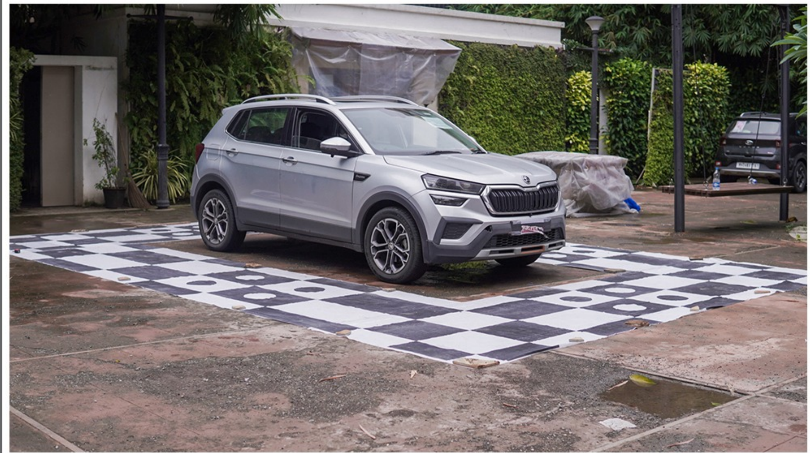
Step 118:- overview of the mat setup - equally alligned on all 4 sides (put small weighted object on the mat in order to restrict movement of the mat)
