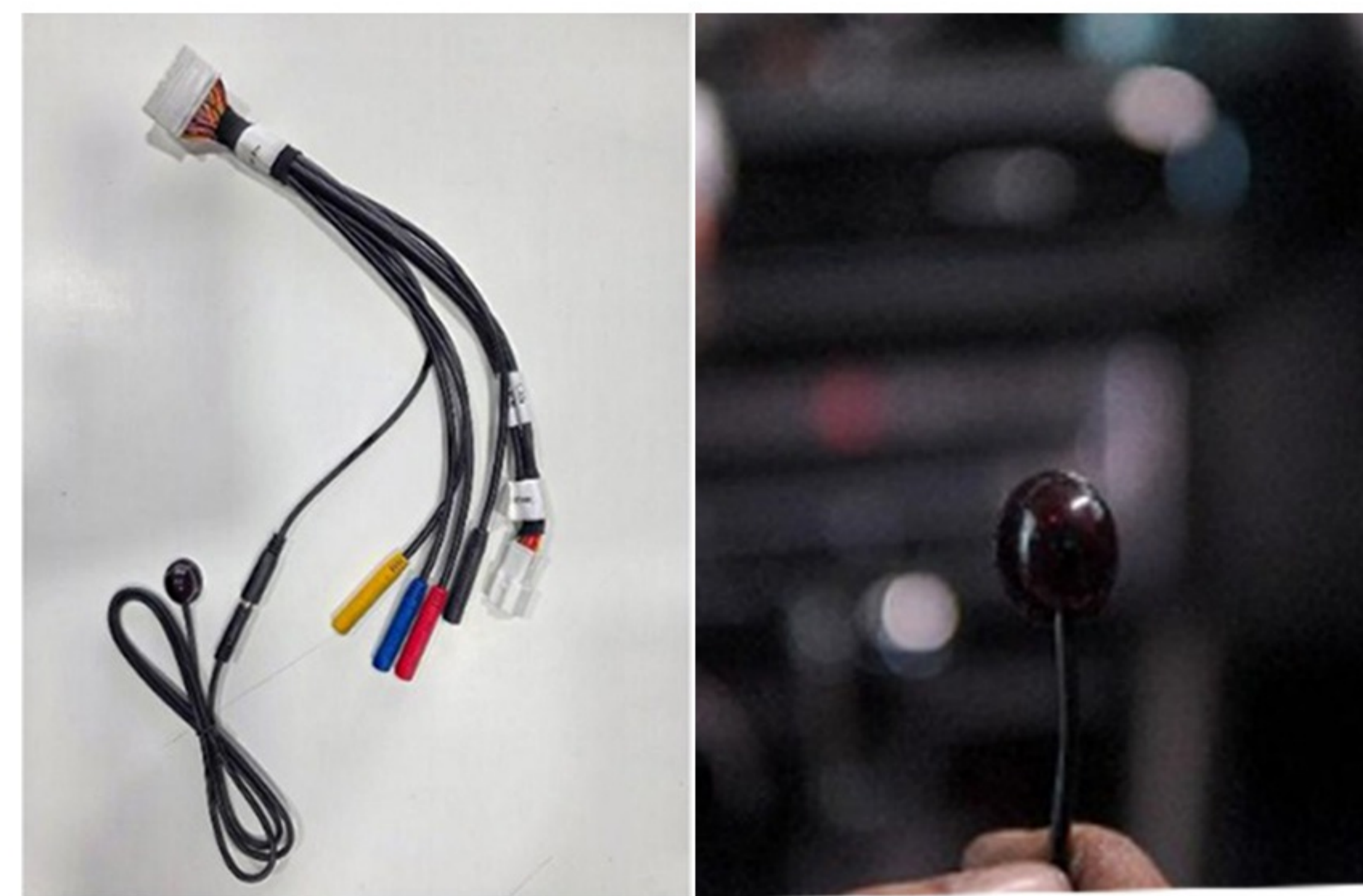
Step 93:-Connect the Remote Sensor to the 32Pin power cord as shown After connecting the sensor cable, pass the cable
