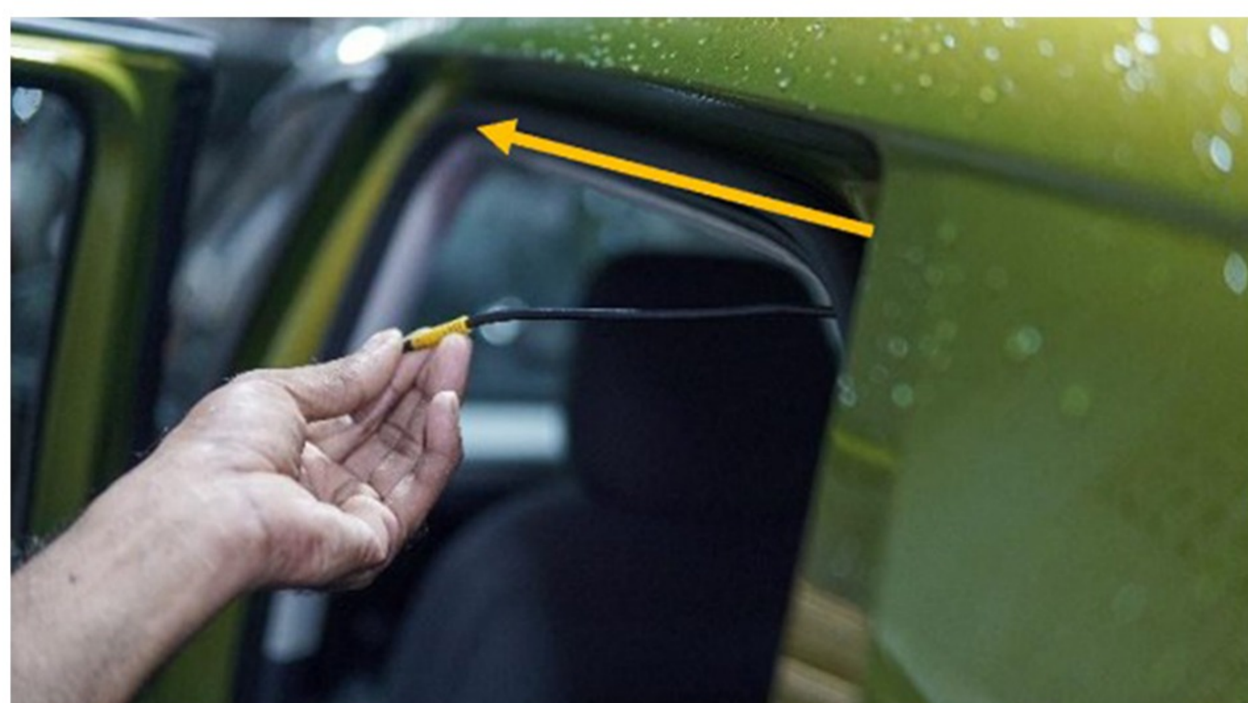
Step 71 :- Routing cable through the Roof liner from rear door to front door.
