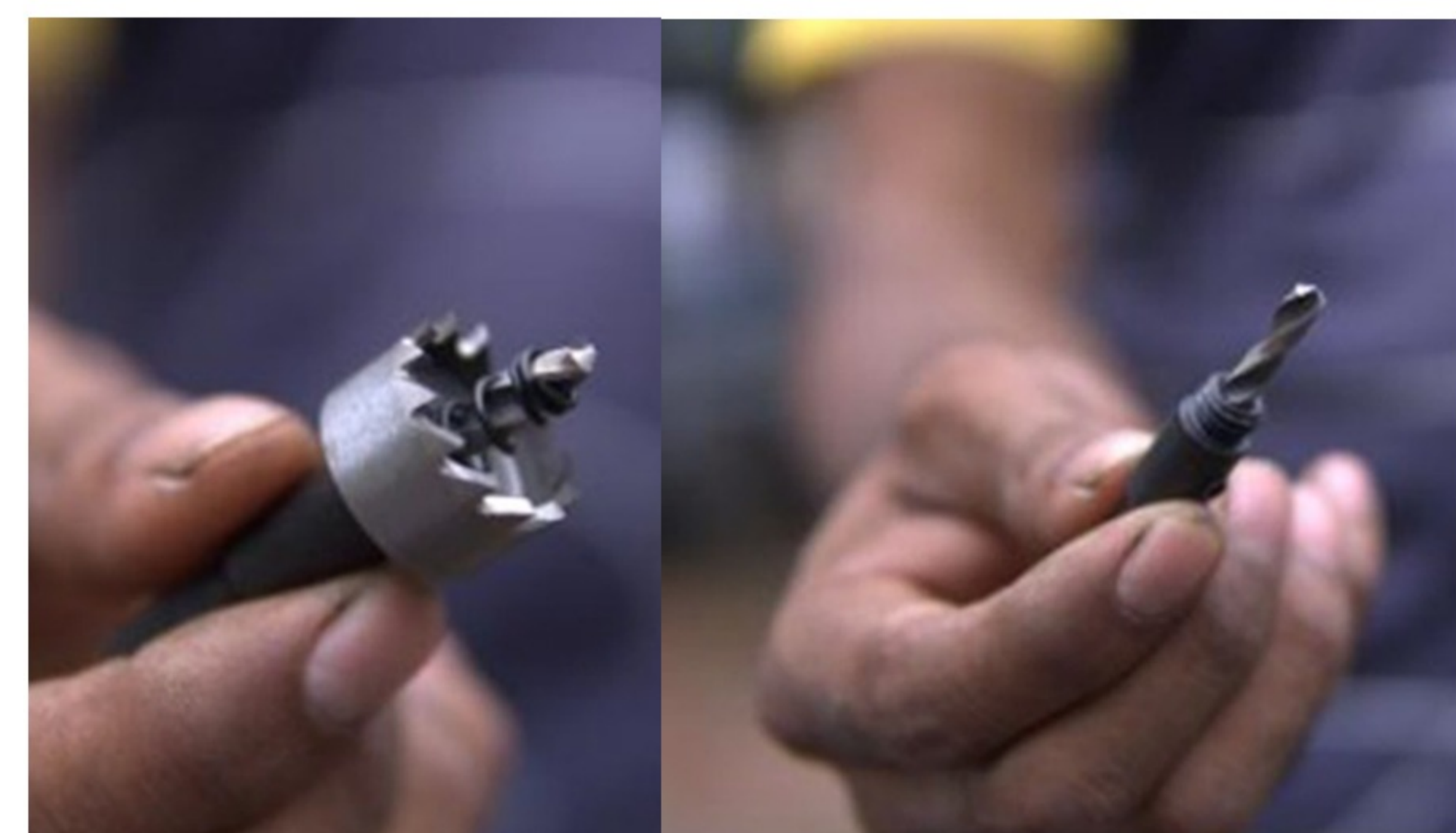
Step 96 :- After removing the 22.5mm bit (Part no 13 ), a smaller bit 8 mm is revealed, place it on the drill machine
