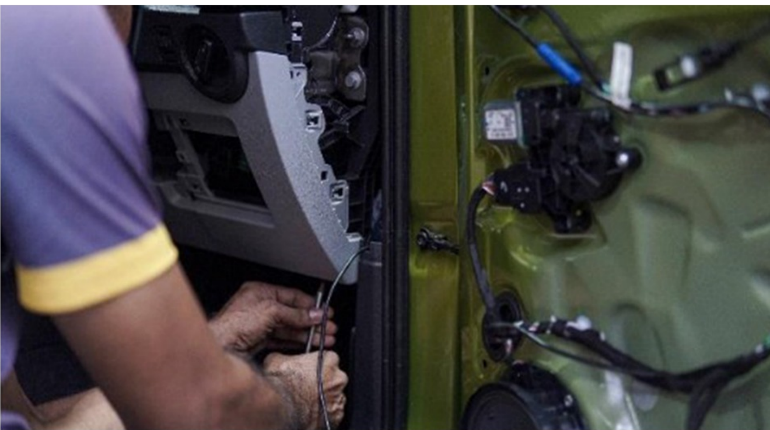
Step 53 :- Remove the fuse box cover as per series process
