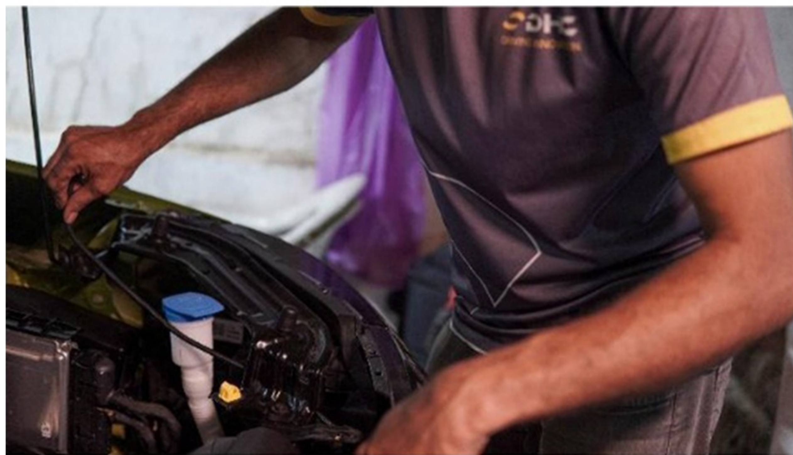
Step 86 :- Route Cable through the edges of engine bay
