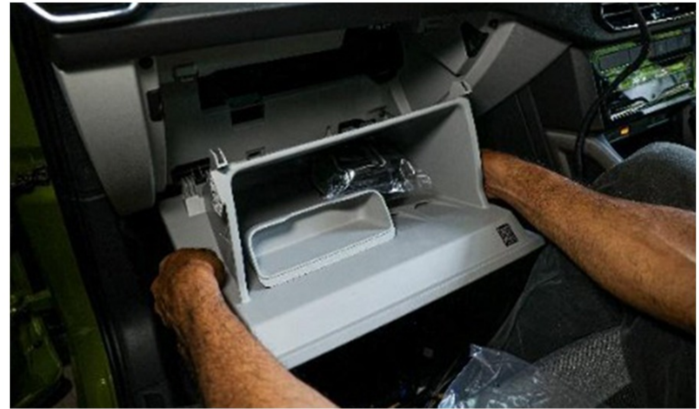
Step 18:-Open glove box as per Series Process
