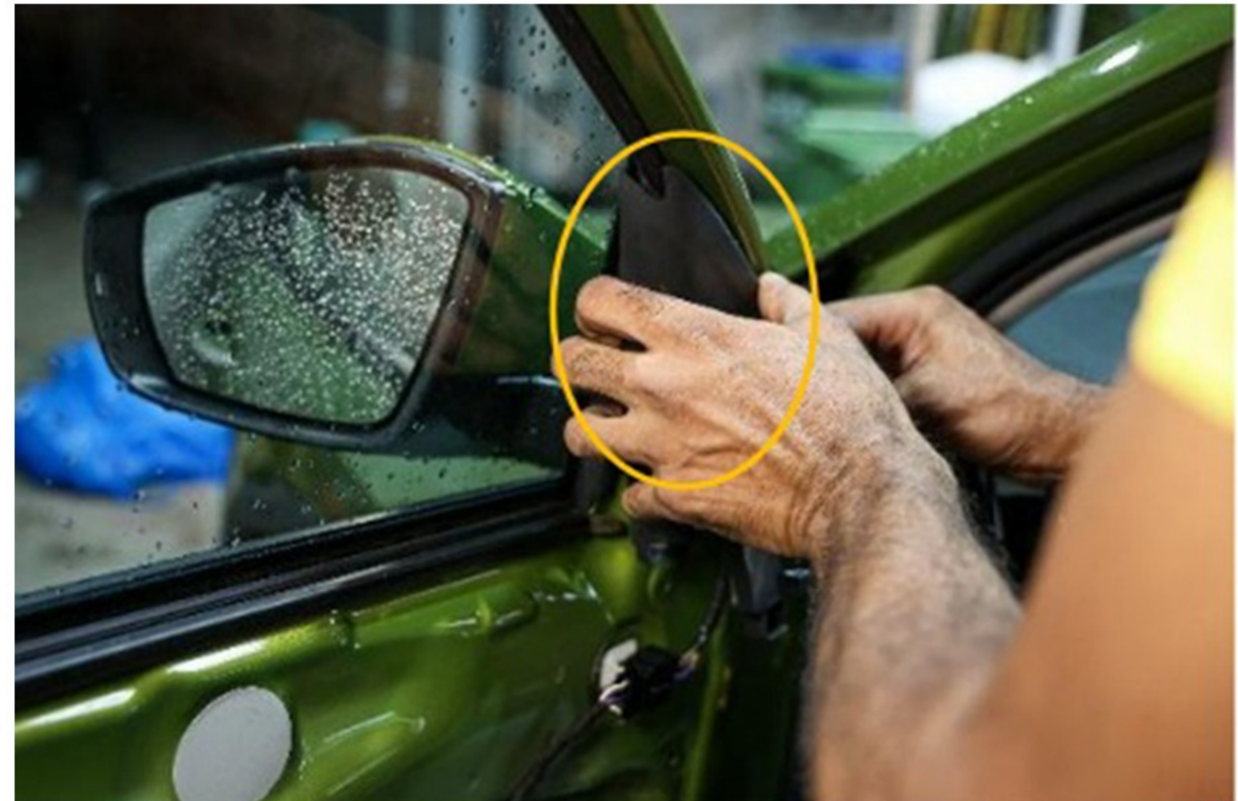
Step 28 :- Remove the left and right ORVM trim Cover as per
