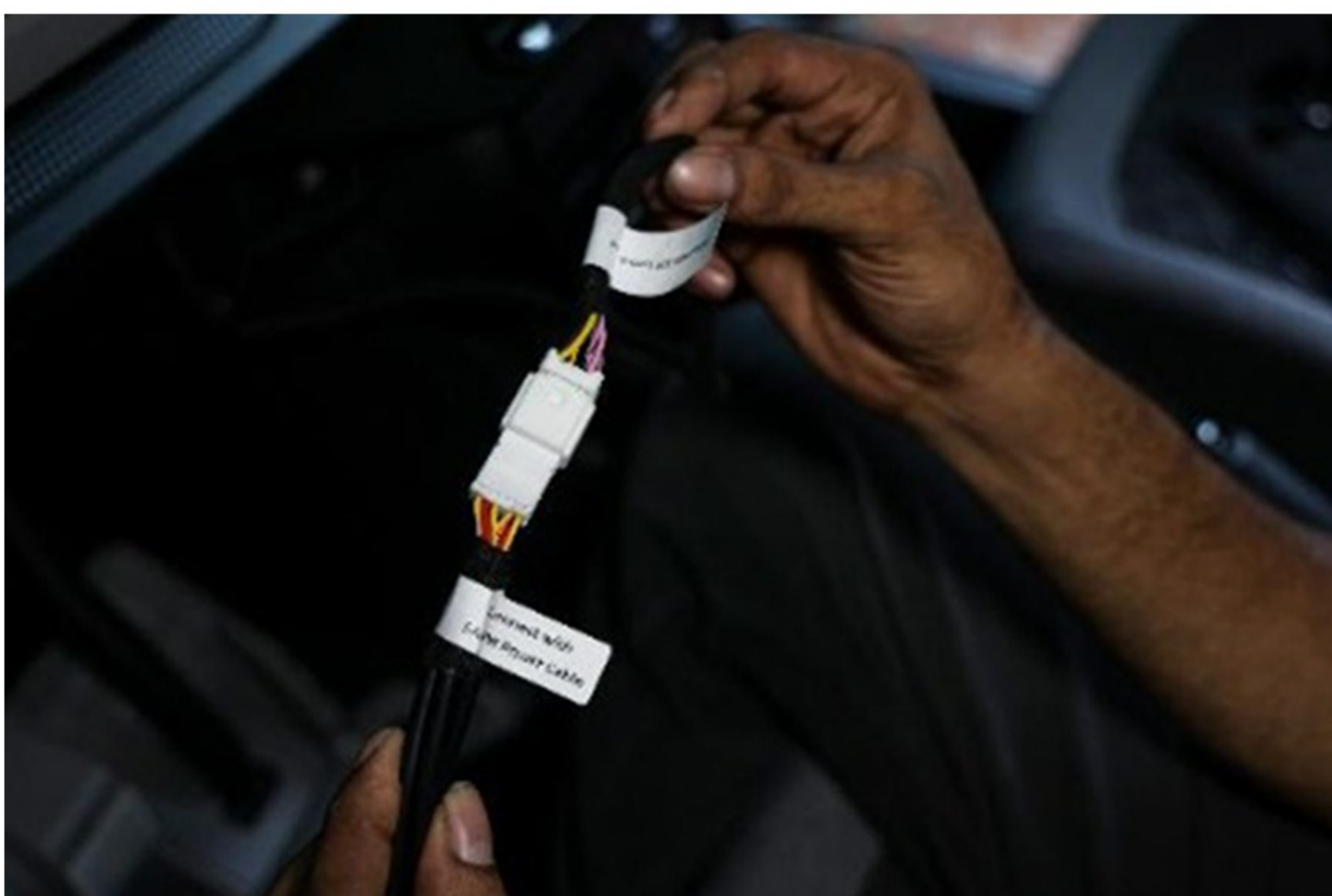
Step 24 :- Connect the 32Pin control cord (part 6 )with SAVW dedicated power cable( part 9) as step 11
