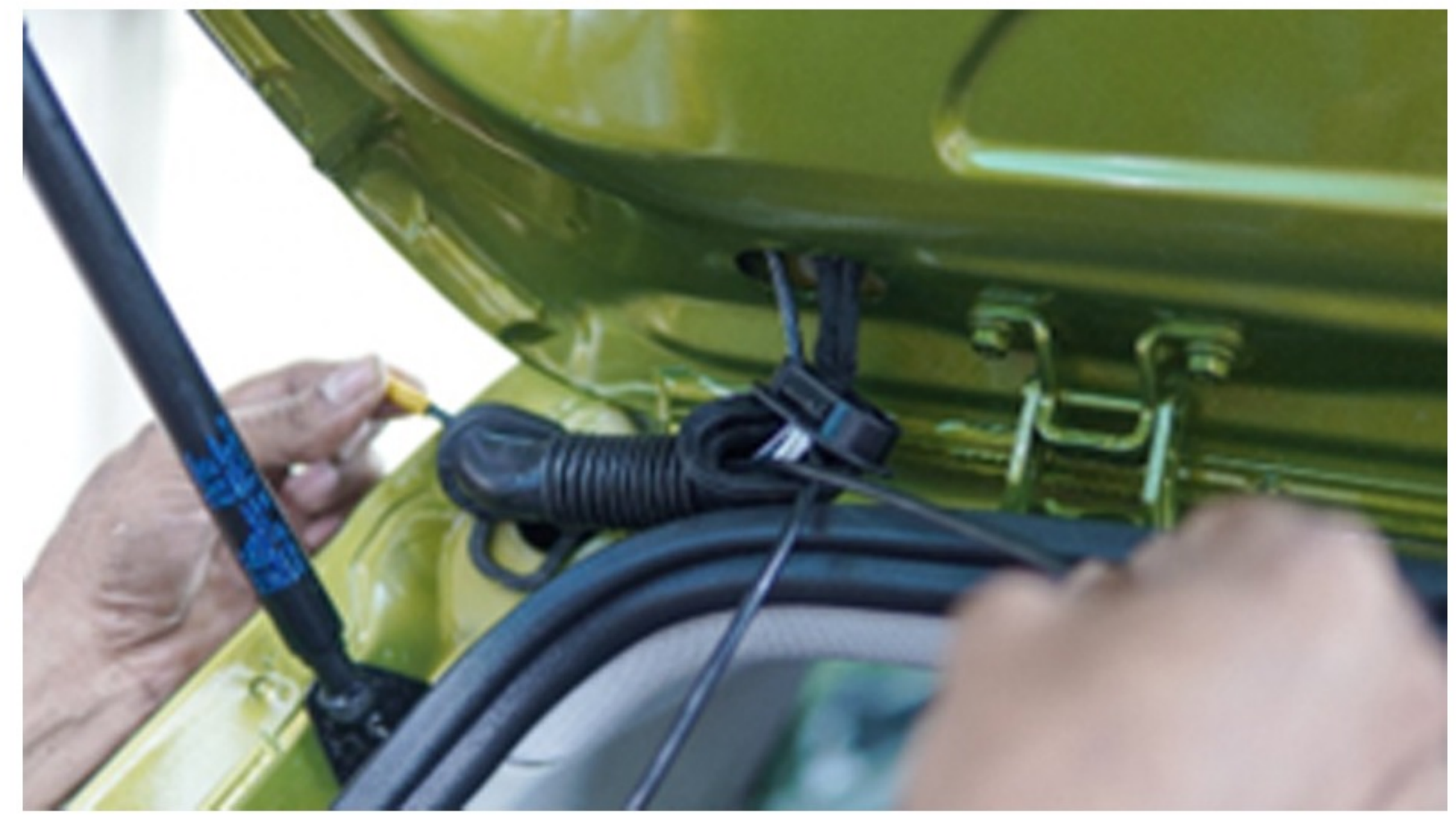
Step 66 :- Route Cable as shown
