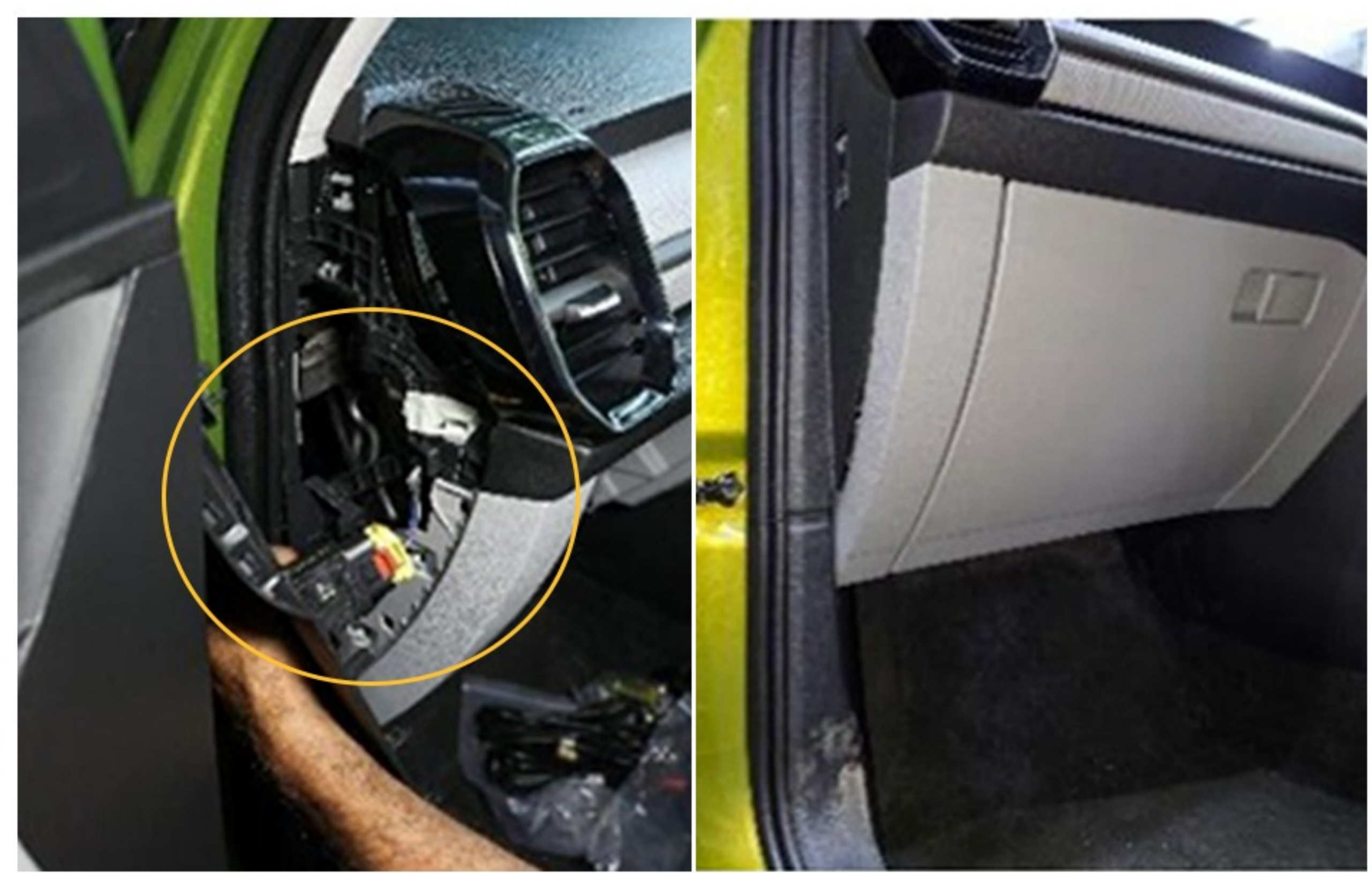
Step 108 :- Reconnect air bag connector & Glove box assembly as par series process
