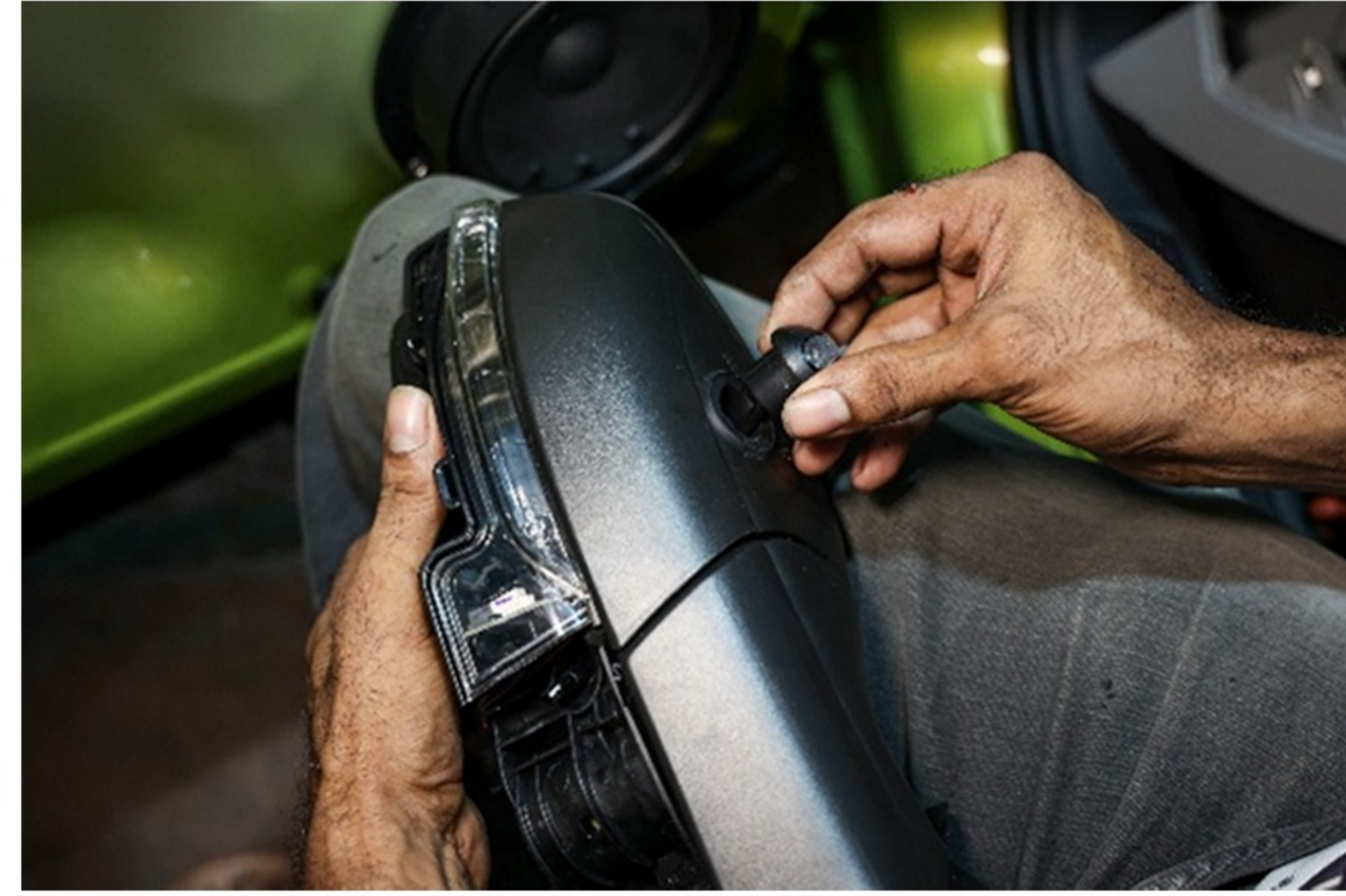
Step 34 :- Insert Left and Right camera in ORVMS respectively with Rubber cover/ cap on the Camera
