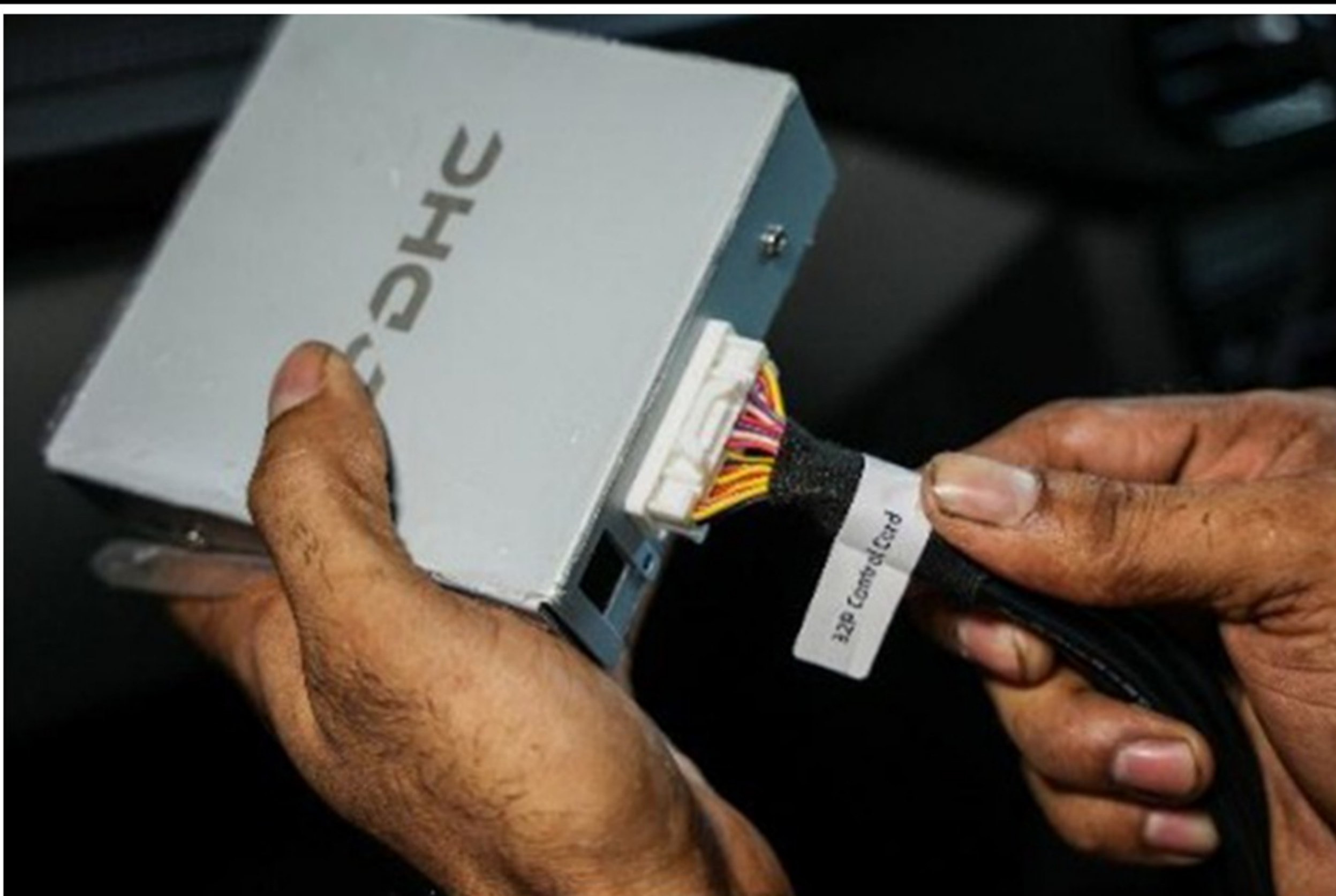
Step 13 :- Connect it to Junction/ECU Box as shown
