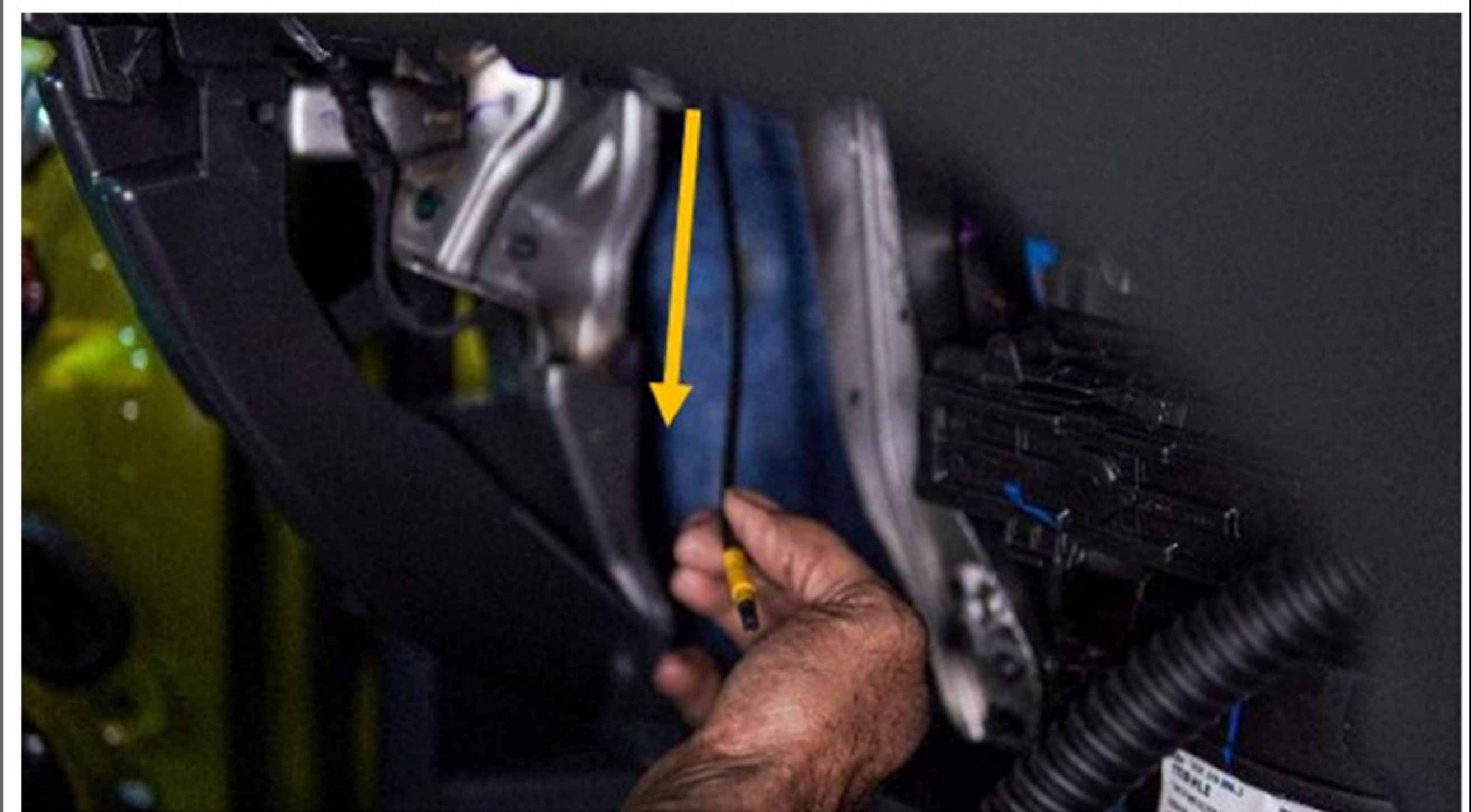
Step 78 :- Bring the cable near the Glovebox area for next connections
