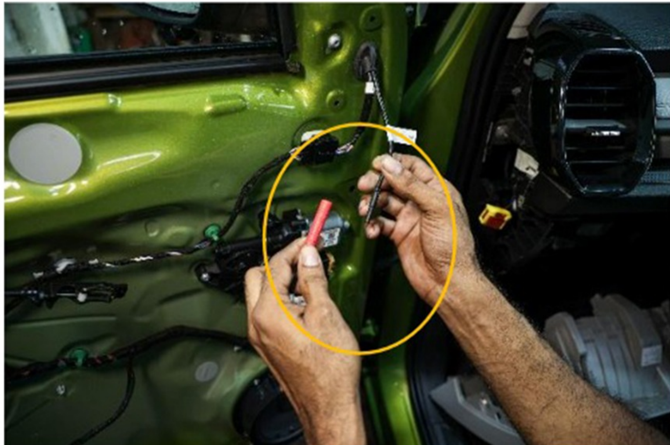
Step 43 :- Connect Left Camera to Left Extension Cable as shown door panel
