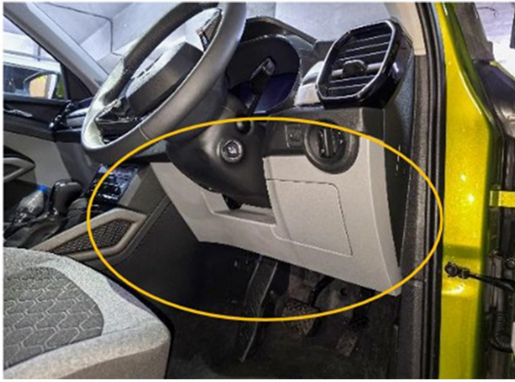
Step 57 :- Assemble fuse box cover back the as per Series process.
