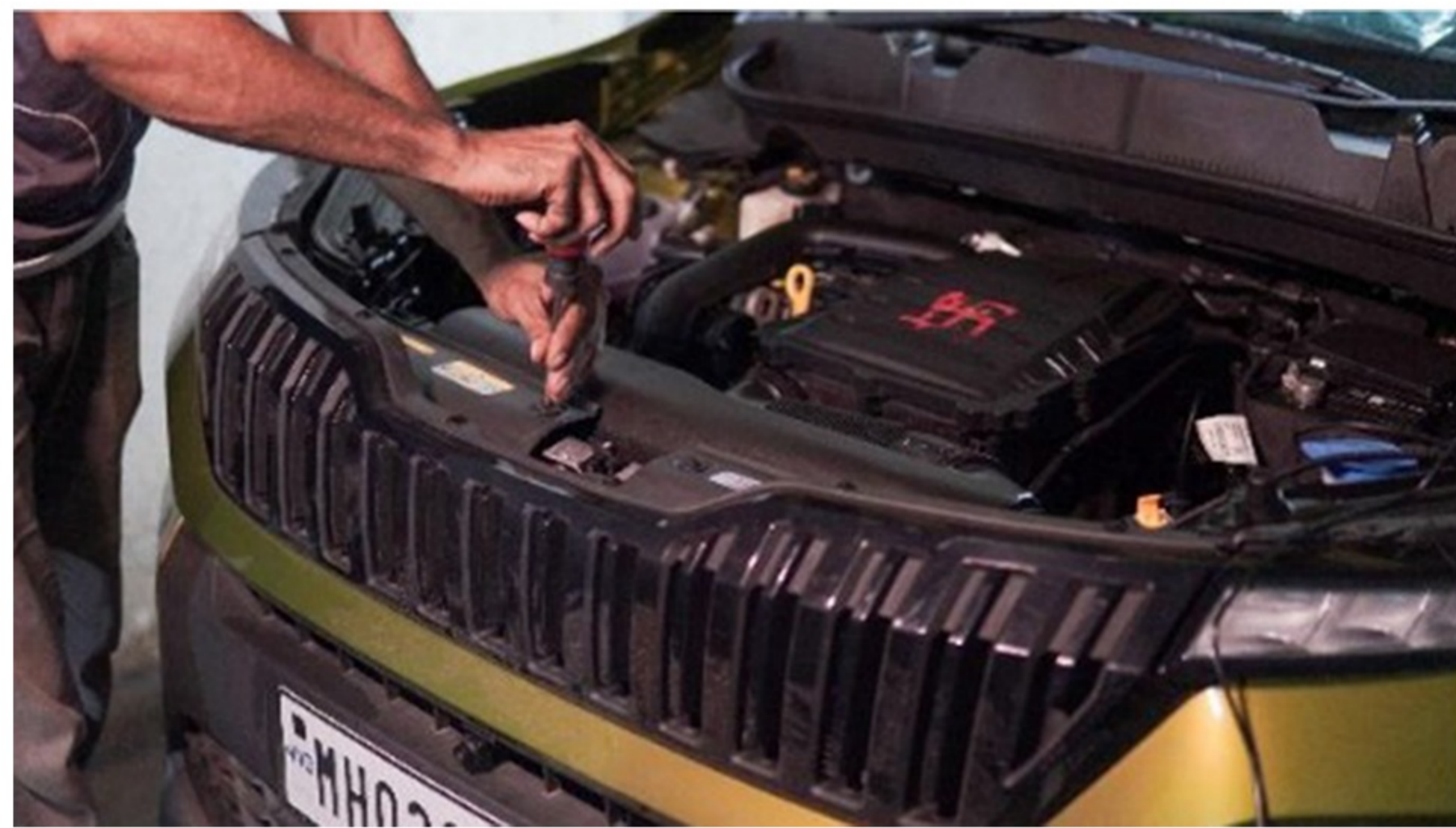
Step 92 :- Reinstall the bumper insert cover near engine bay as per series process
