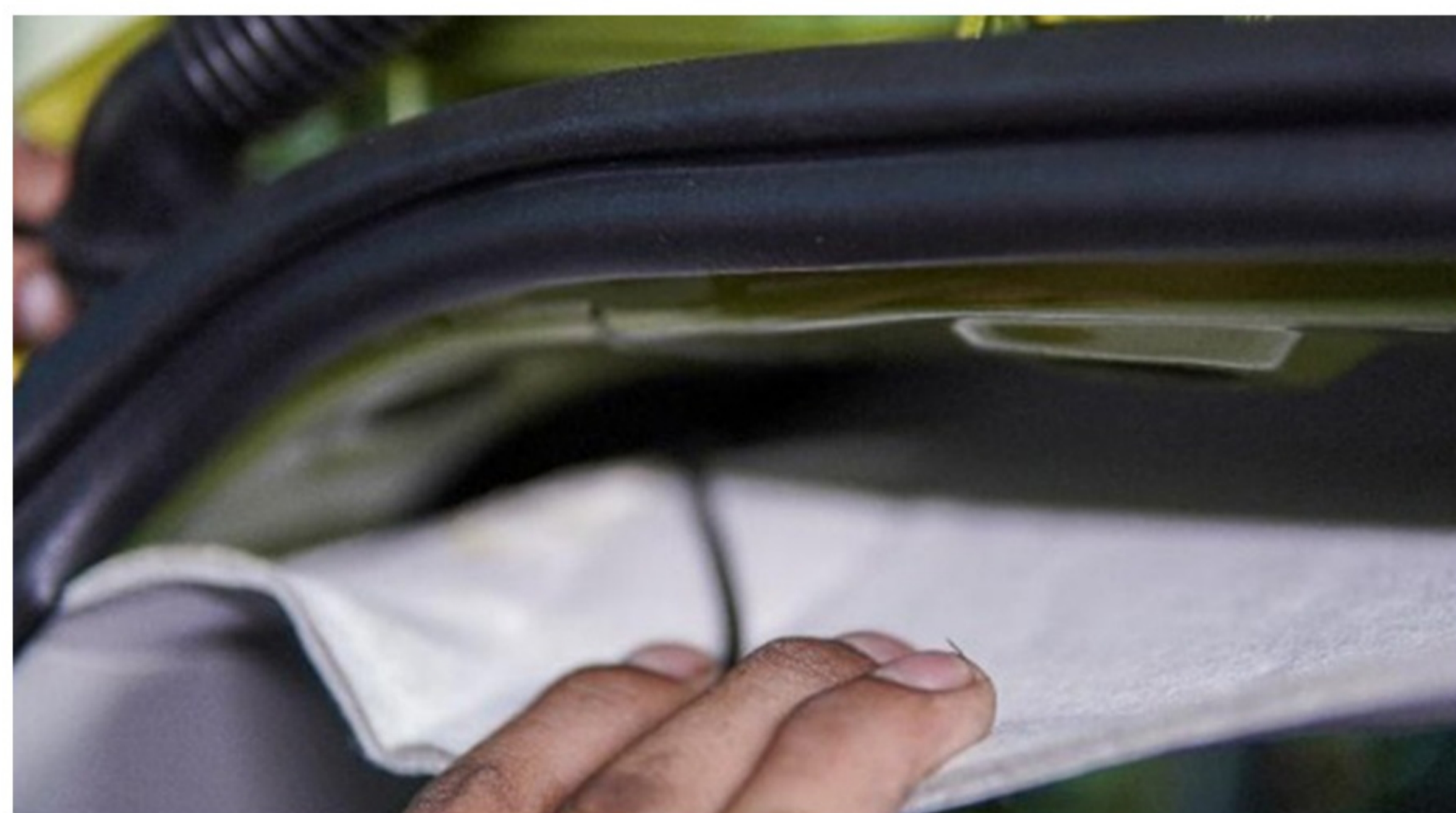
Step 69 :- Remove roof liner gently and routing of cable through roof liner.
