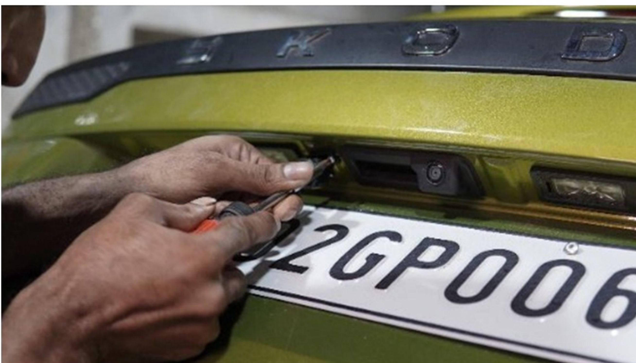
Step 101:- Screw(Part no 12) and fix the rear camera (Part no 7)
