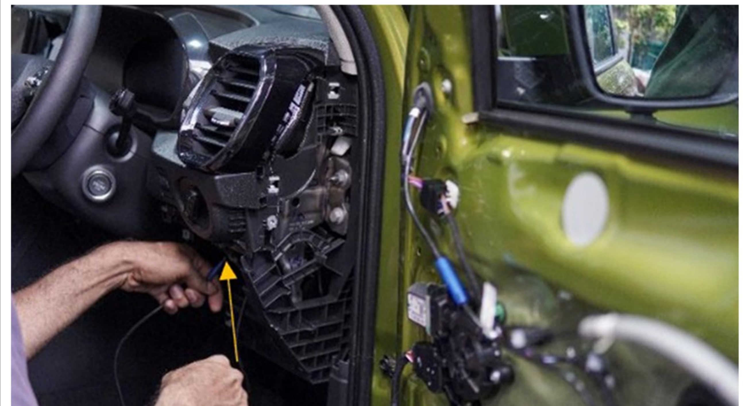
Step 54 :- Route the Cable as shown
