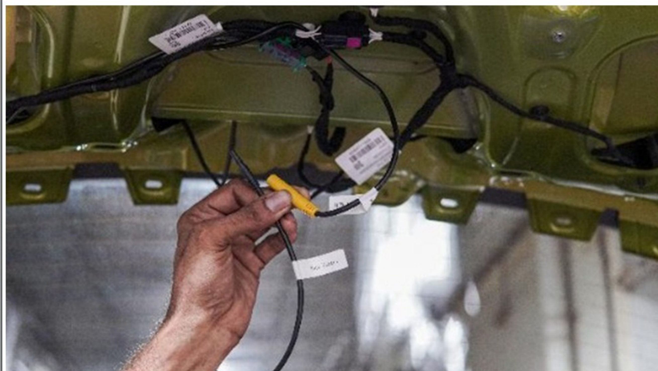
Step 102:- Connect rear camera (Part no 7) to the rear extension cable (Part no 4)
