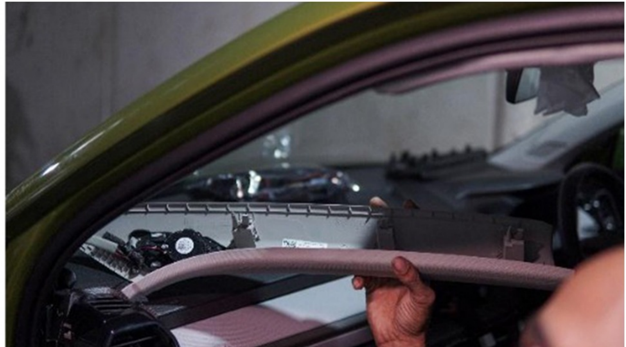
Step 75 :- Dismantle A pillar trim as per series process
