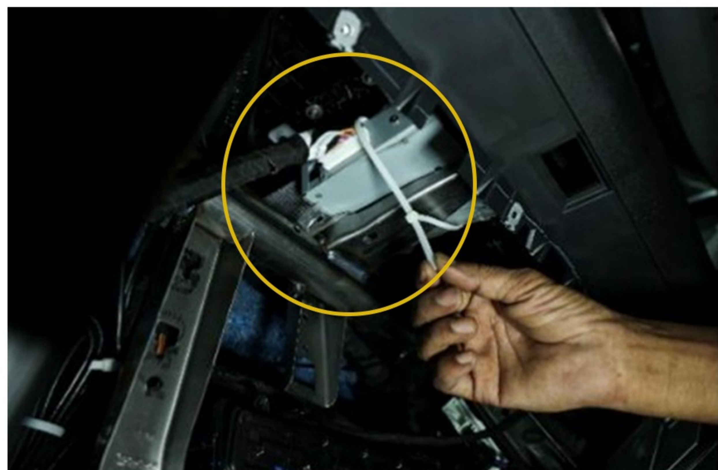
Step 107 :- Place the junction box ( Part no 1) as shown and tie it with 2 tie cable and ensure secure fittment
