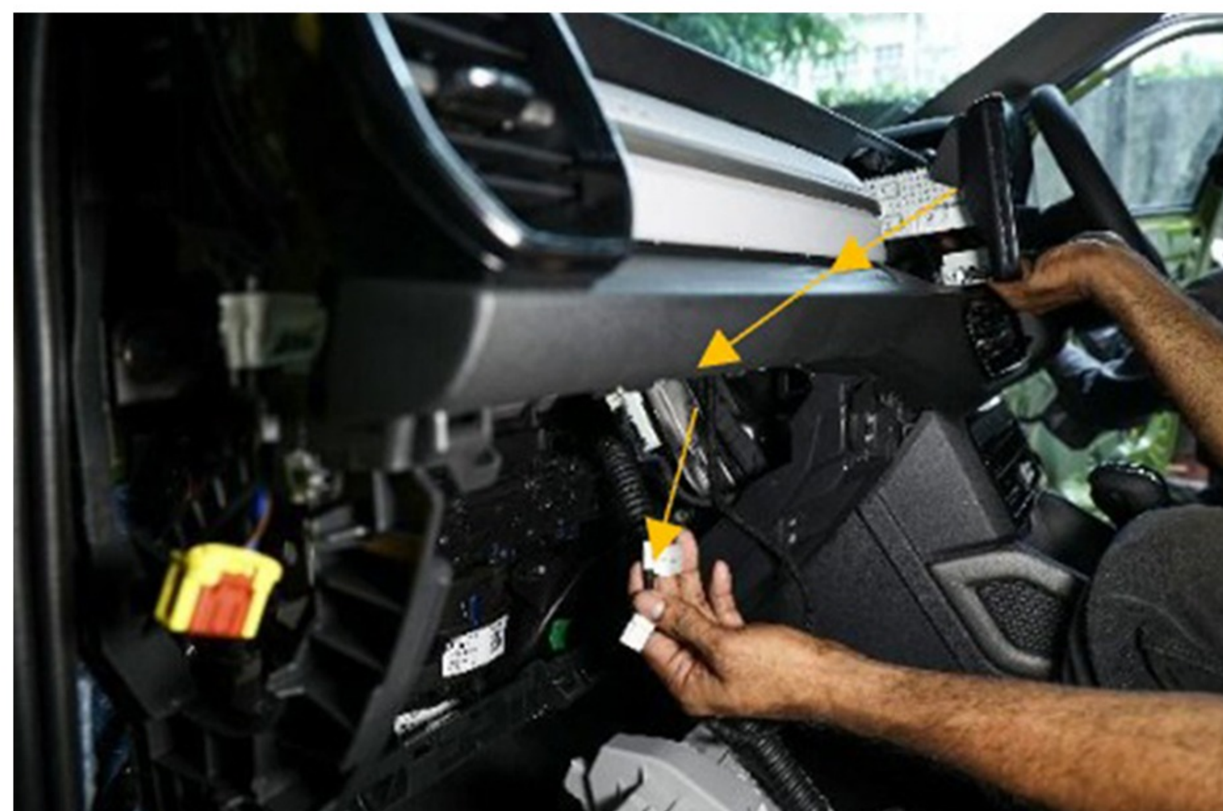
Step 23 :- Route the cable from back of multimedia to glove box area as shown
