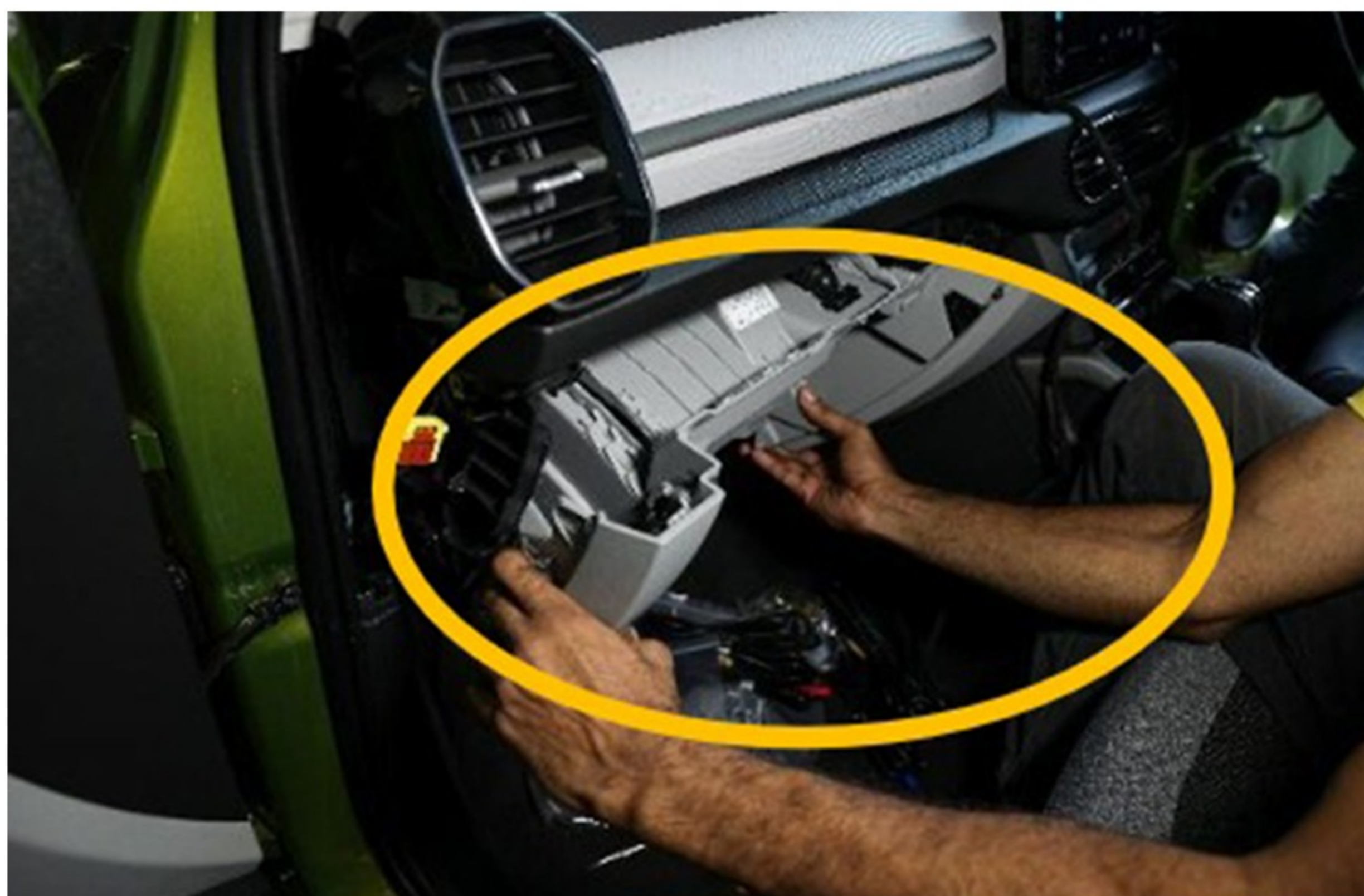
Step 22 :- Remove the glove box assembly
