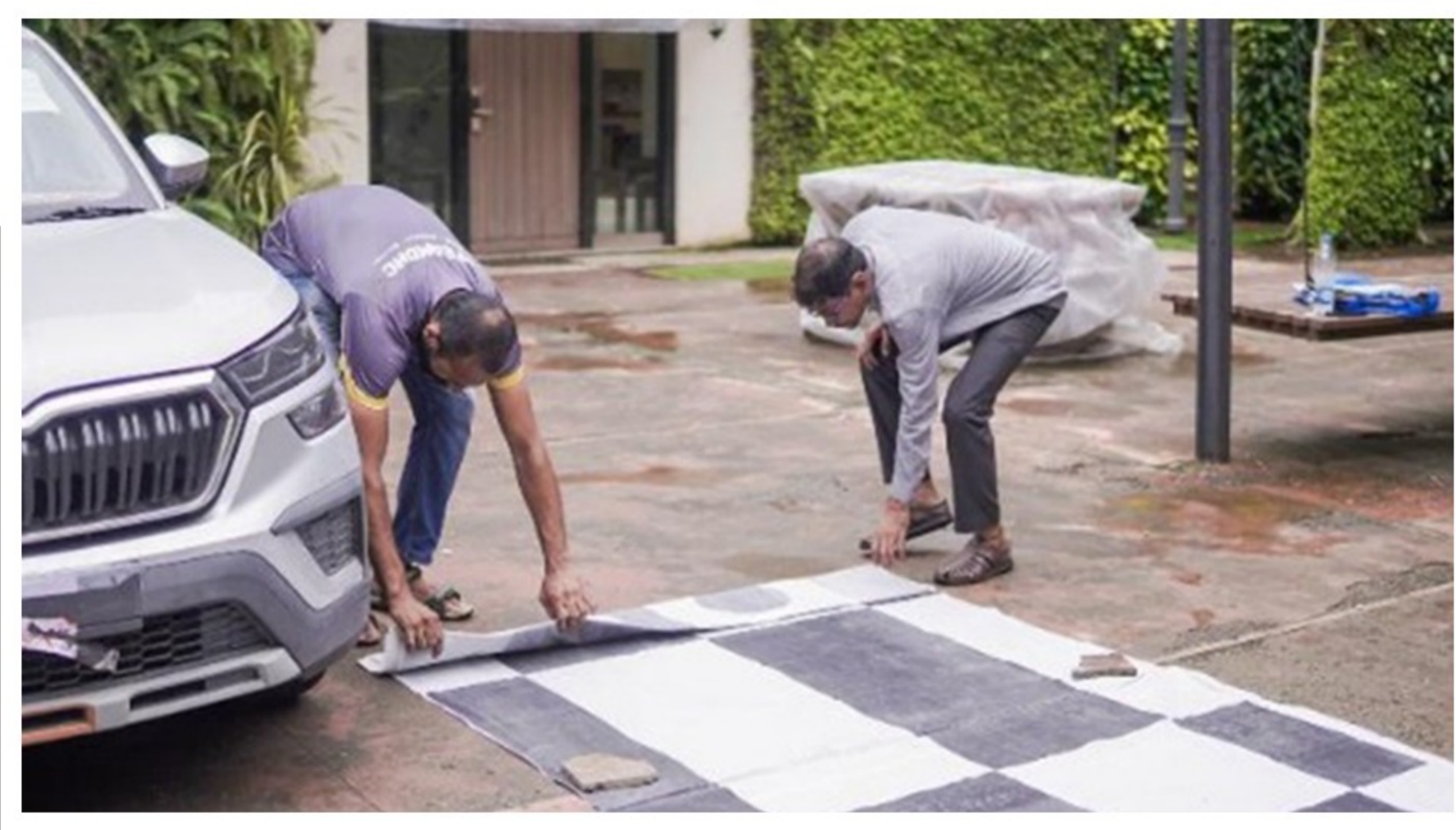
Step 114 :- Place the mat carefully in orderly way to the right side of the car, the mat should remain staright/ parallel to car
