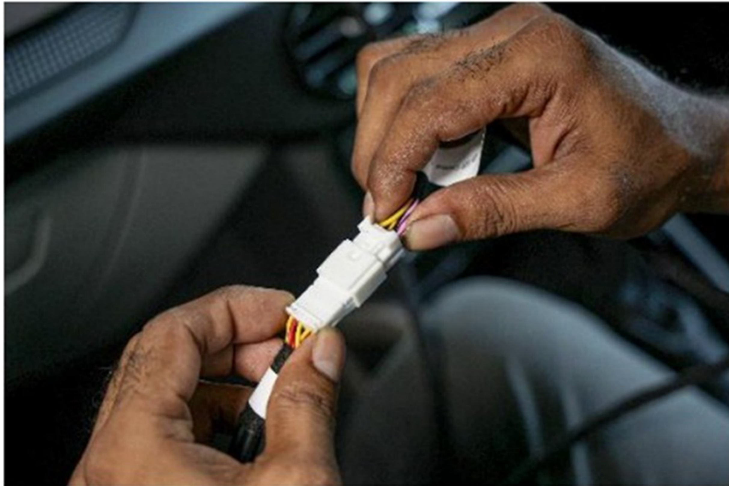
Step 11 :- Connect the 2 sockets as mentioned on the part stickers
