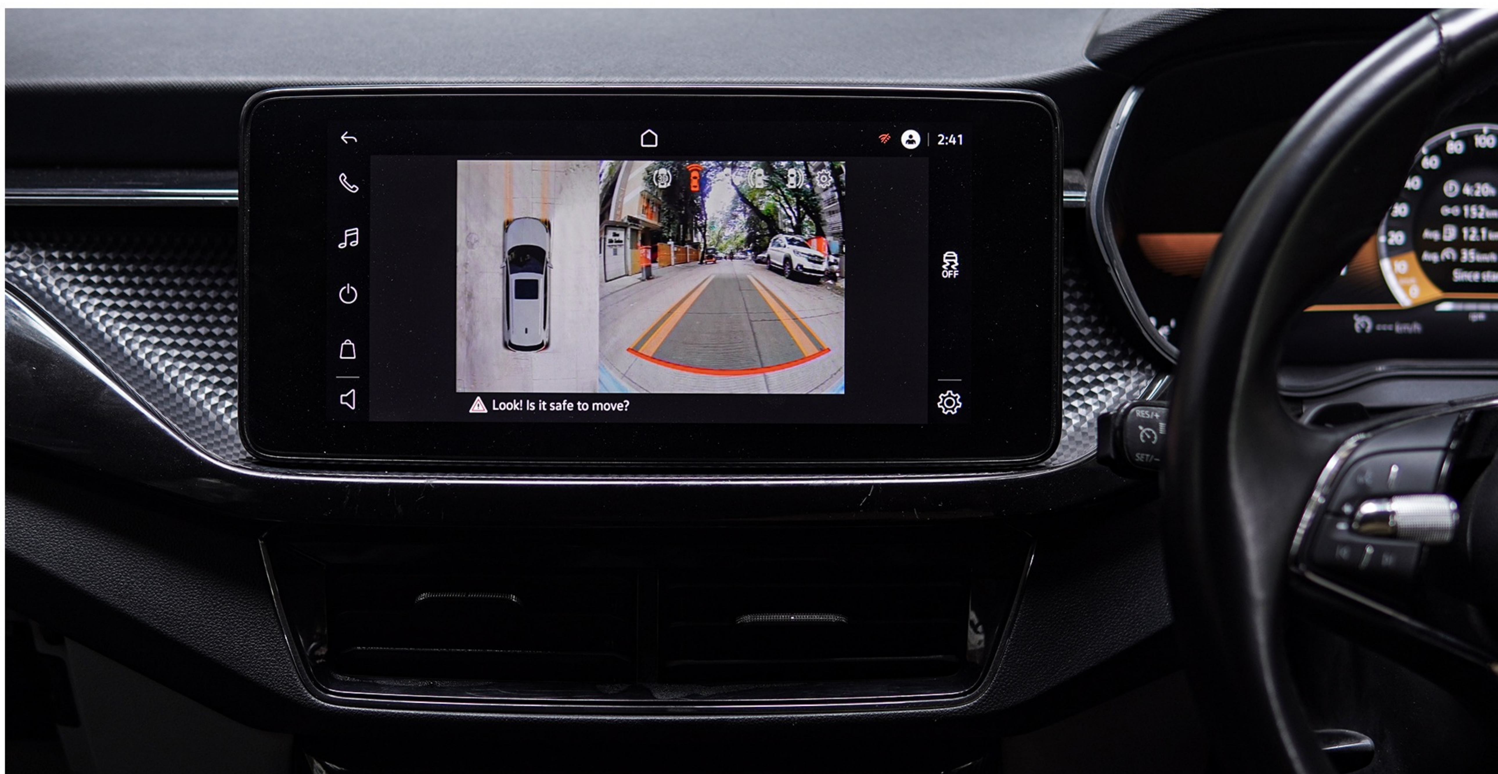
Step 131 :- Installation Completed, take a test drive to test the dynamic guidelines and calibration
