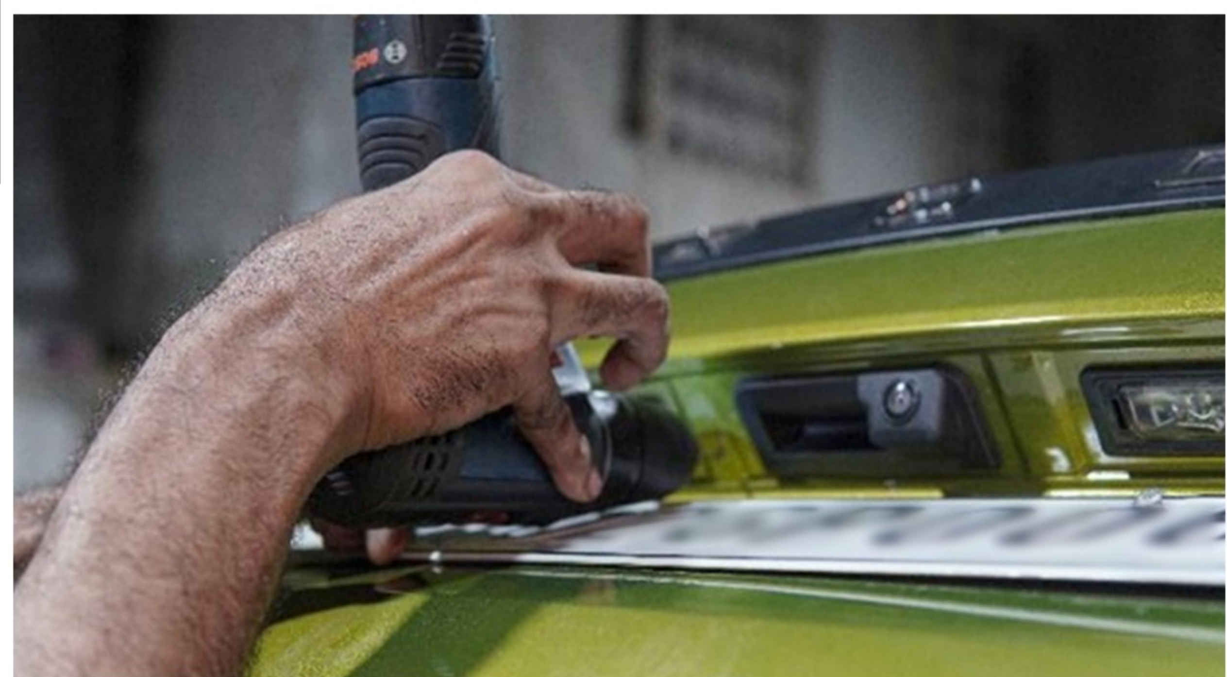
Step 98 :- Drill a hole as per marked location in step 95 paint touch up to be done to avoid rusting if required
