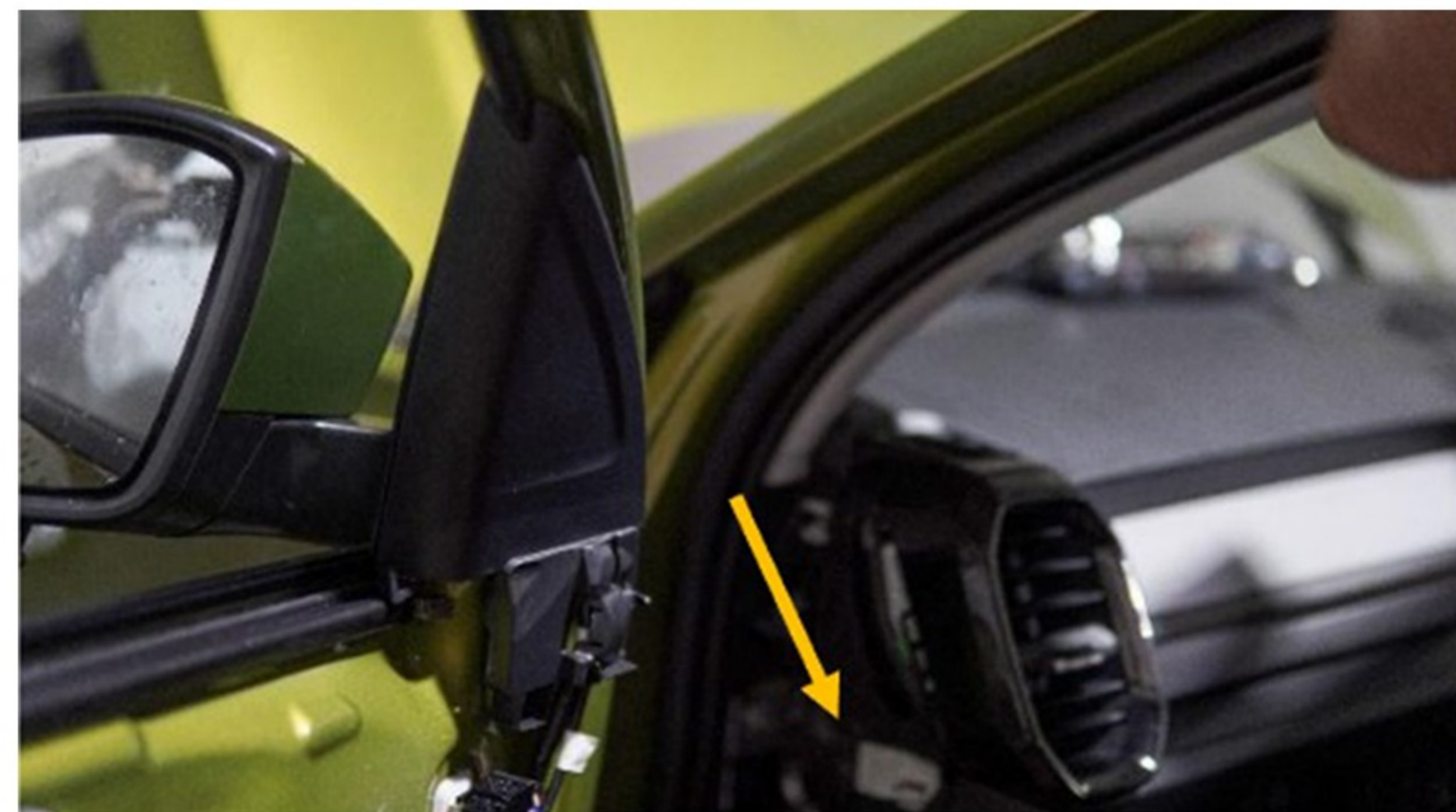
Step 77 :- Route the cable through dashboard side trim and refitment of A pillar Trim and roof Liner
