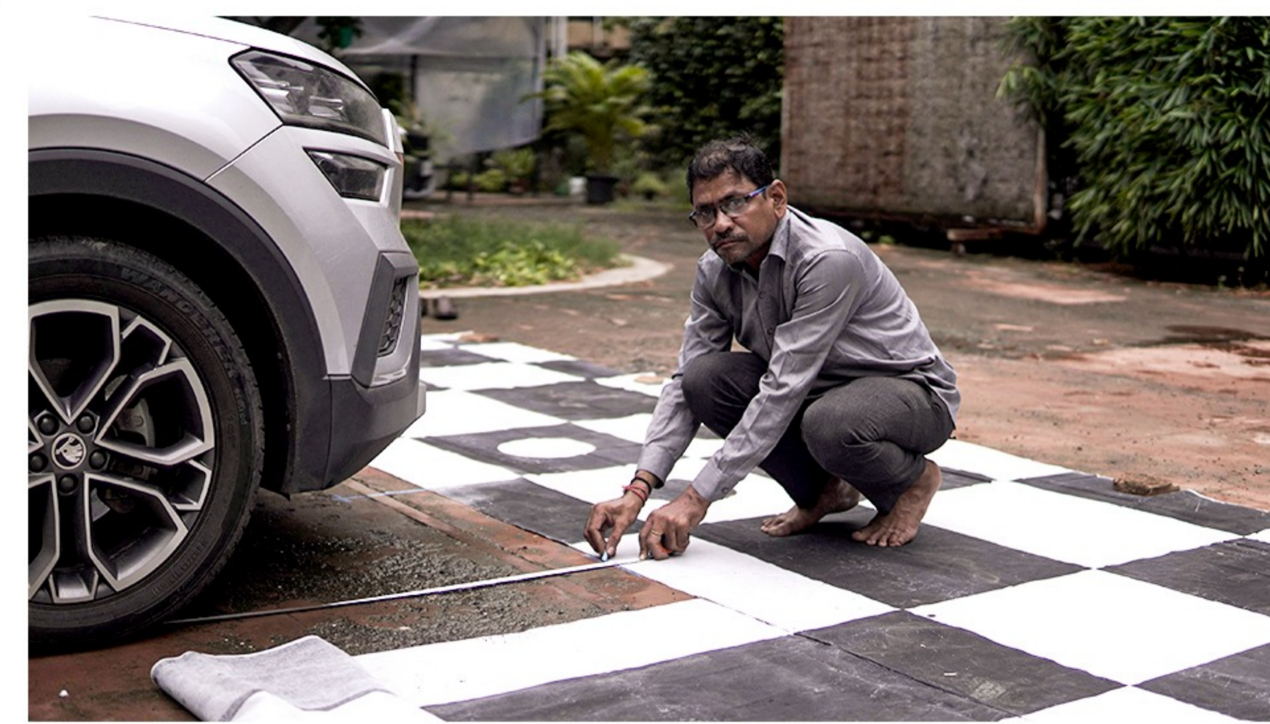
Step 112 :- Measure from the tyre 35 inches and align the mat 35 inches from the both front tyres mat has to be placed. (Please refer to the video for reference.)
