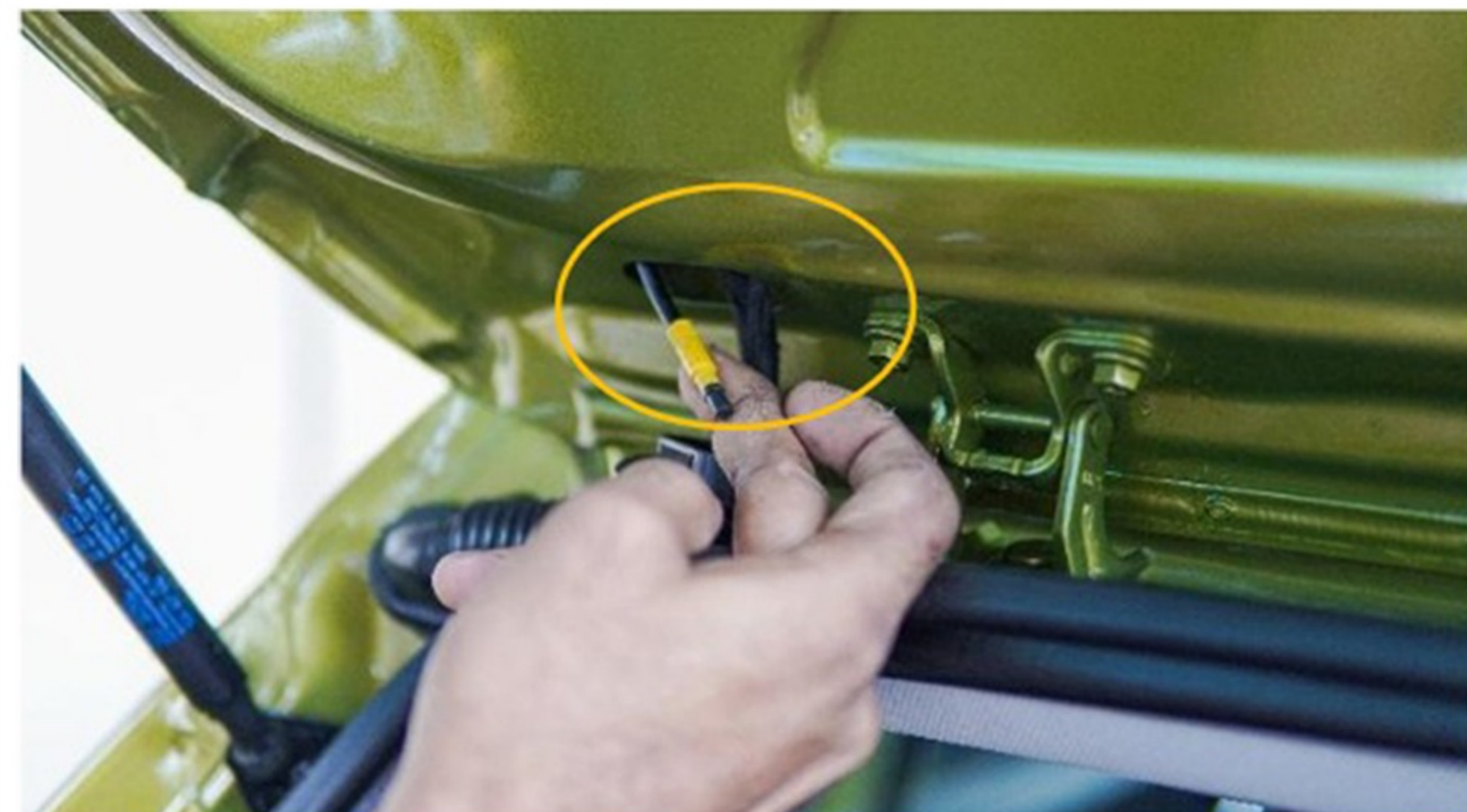
Step 64 :- Route Cable as shown from holes in tail gate.
