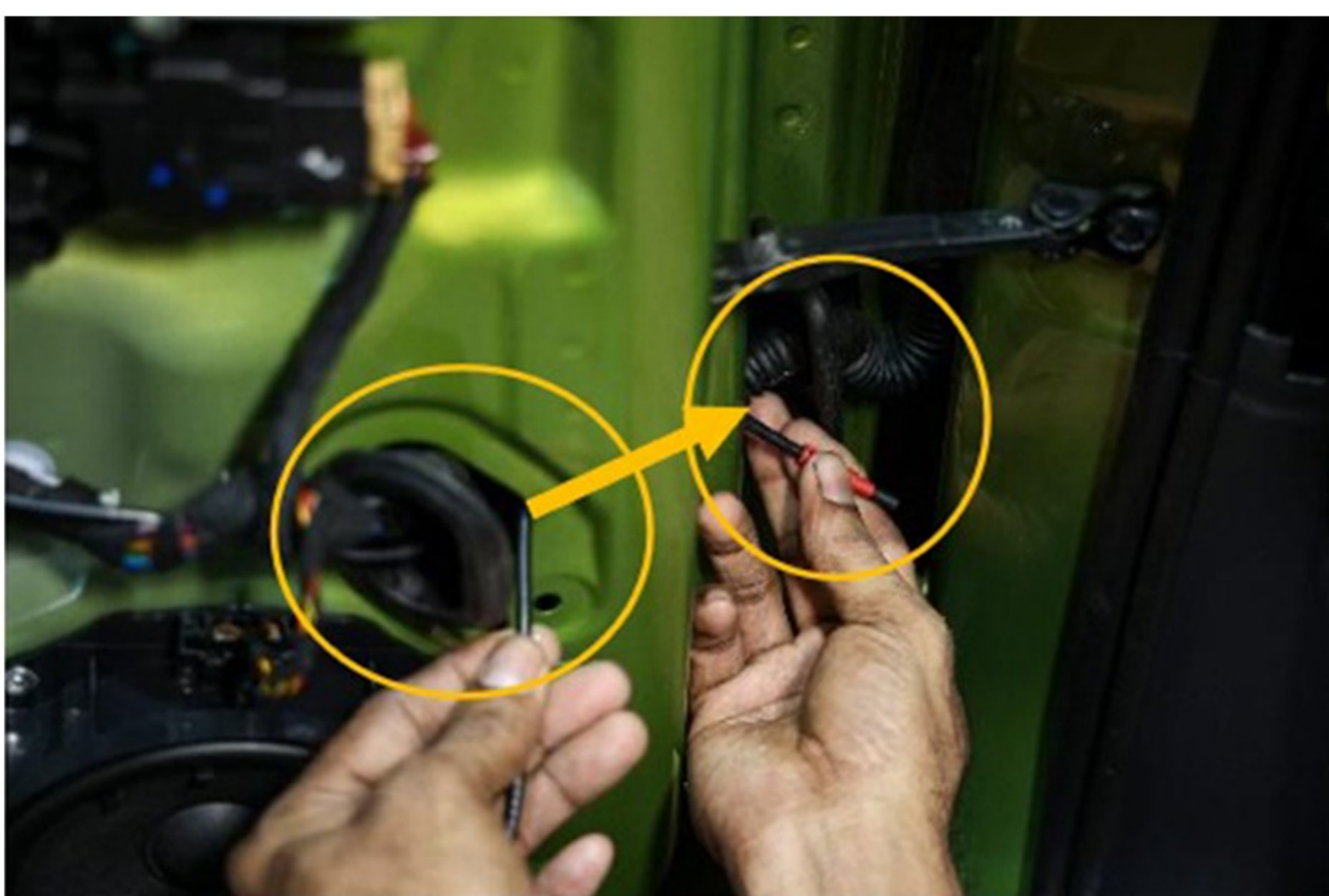
Step 47 :- Route cable from the rubber sleeves to the area shown in the image ( Route delicately)
