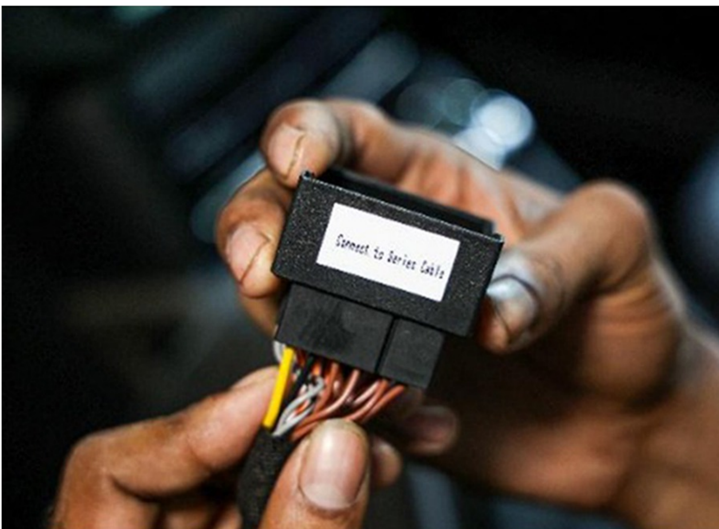
Step 7:- Connect SAVW Dedicated Power Cable (part 9) to Series Cable as per stickers on the part
