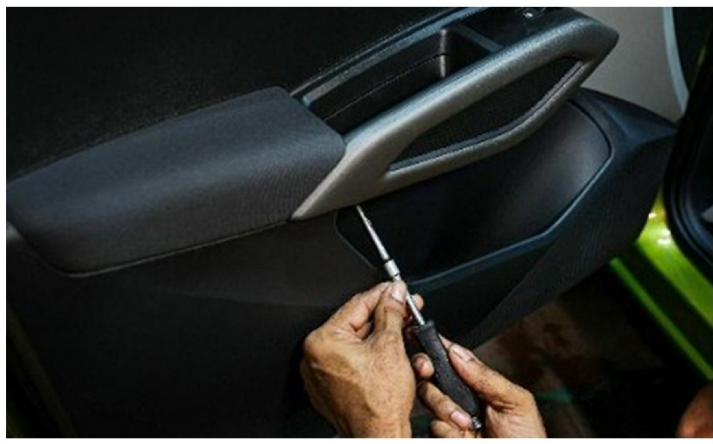
Step 26 :- Remove the door trim as per series process
