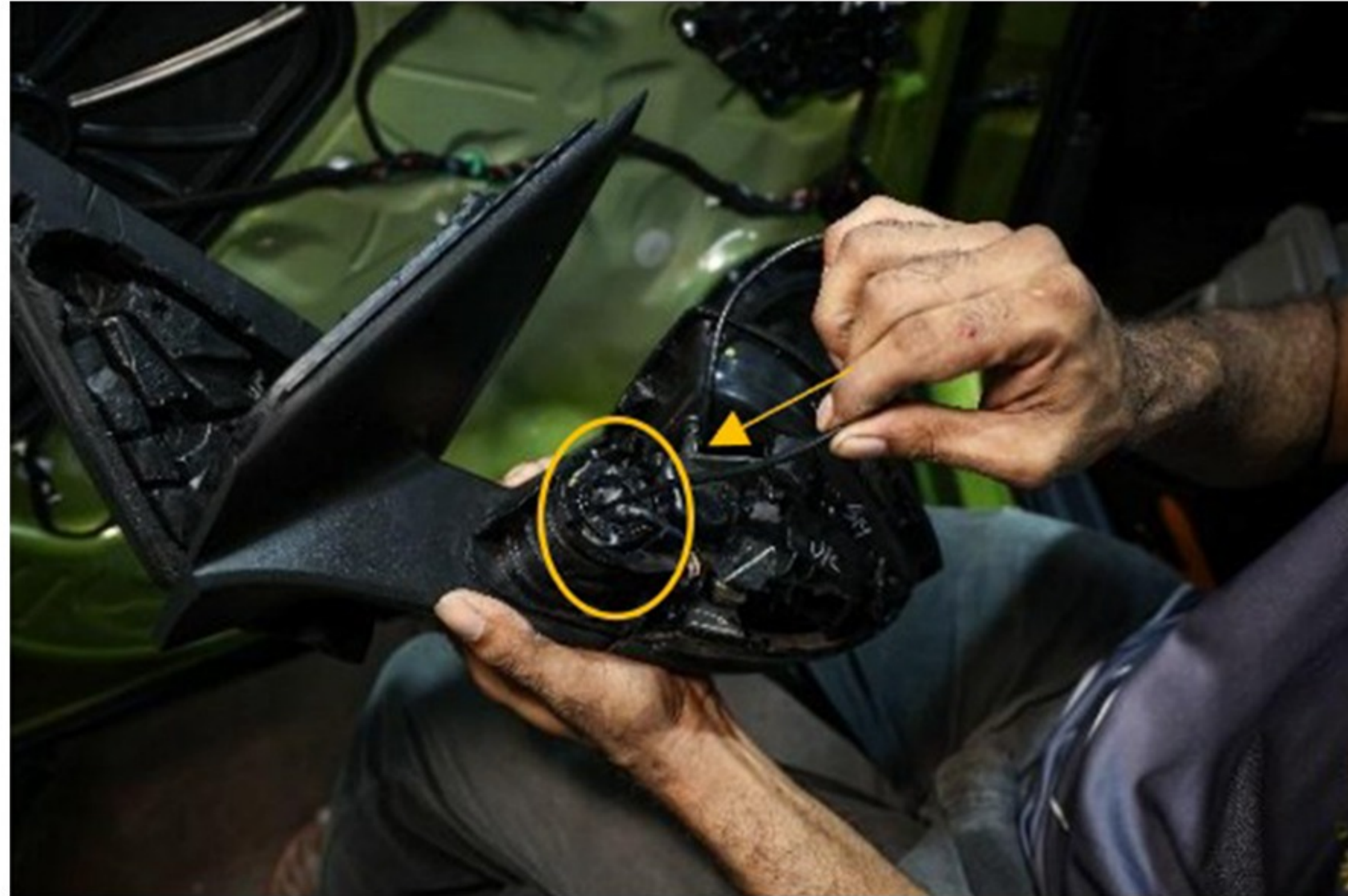
Step 35 :- Route the Cables Through the space marked (for more clear demonstration kindly refer to the installation video)
