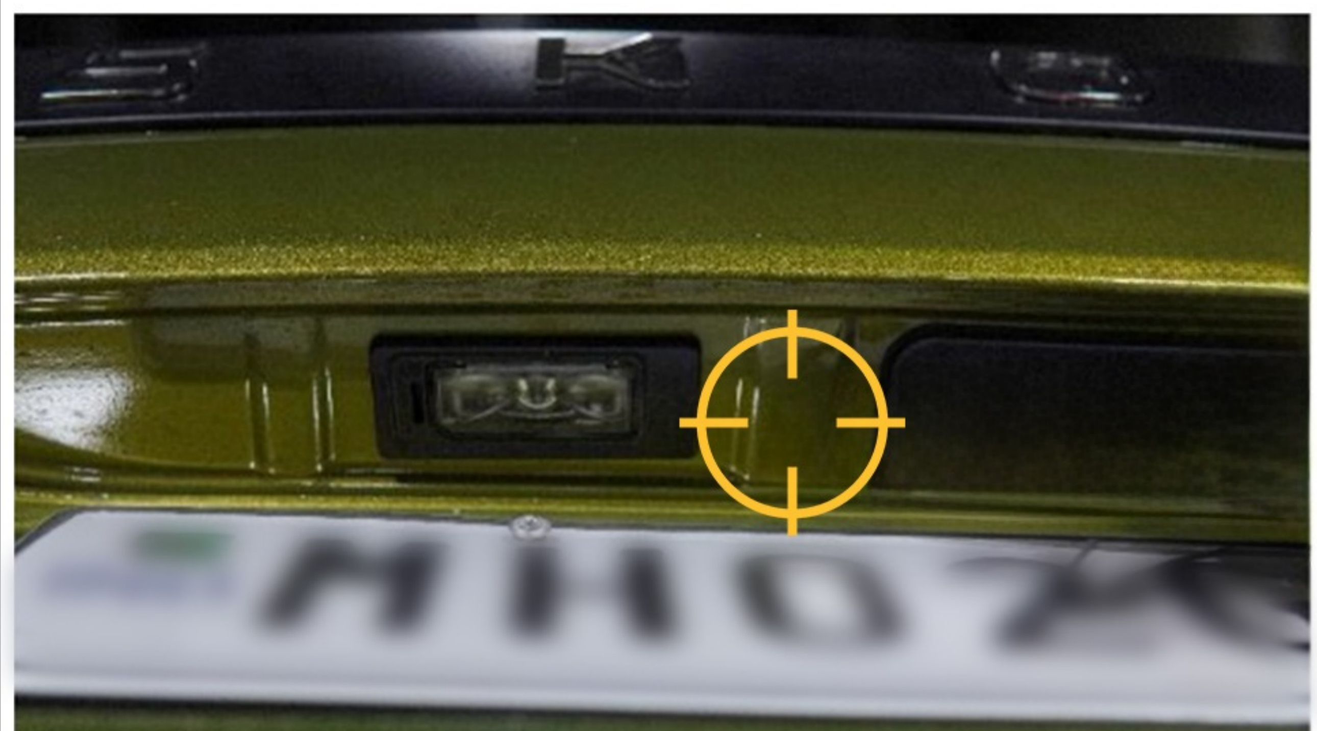
Step 95 :- Measure the length of 1inch from all 3 sides from left boot light to tailgate
