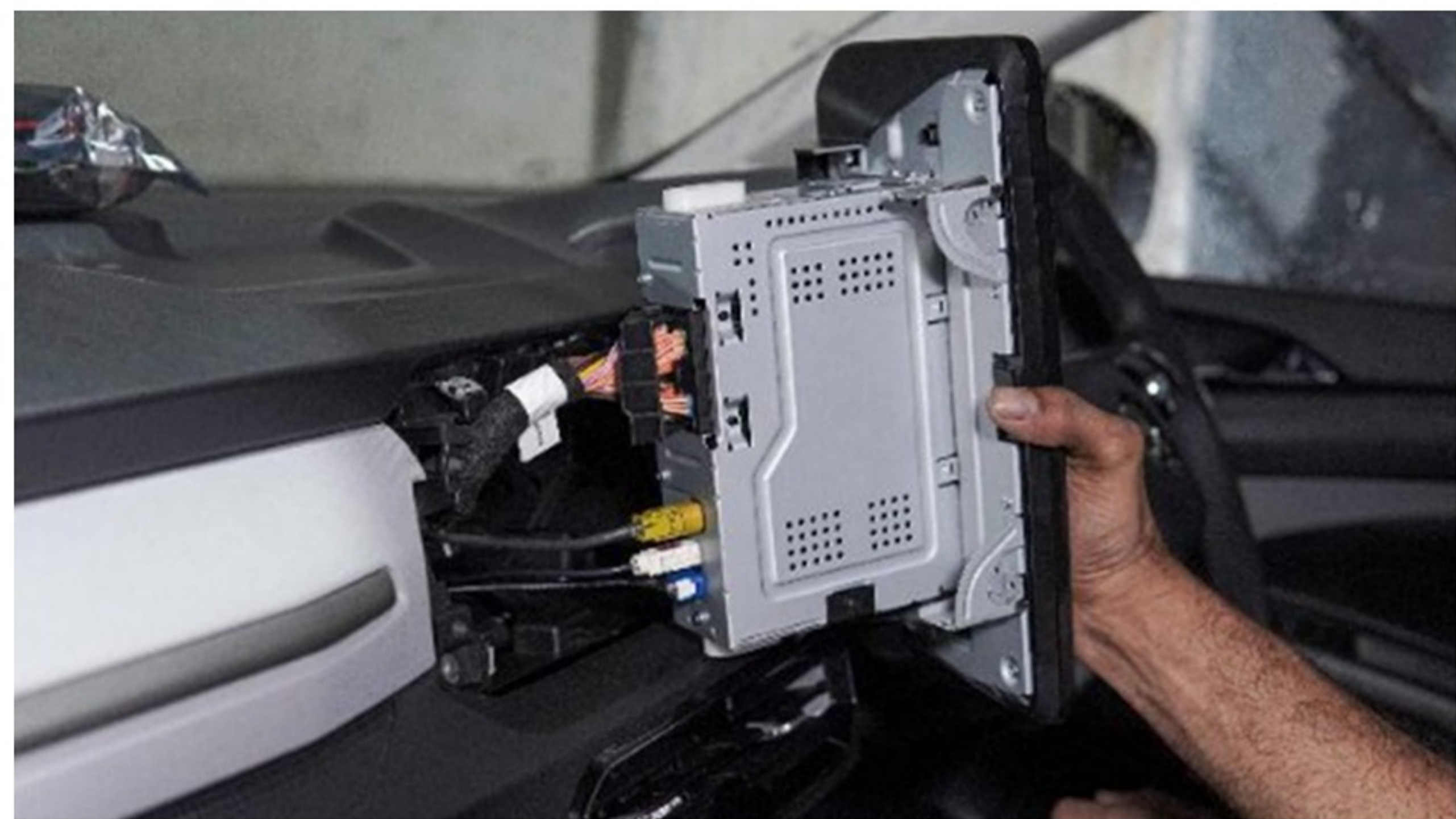
Step 110 :- Connect the multimedia cables
