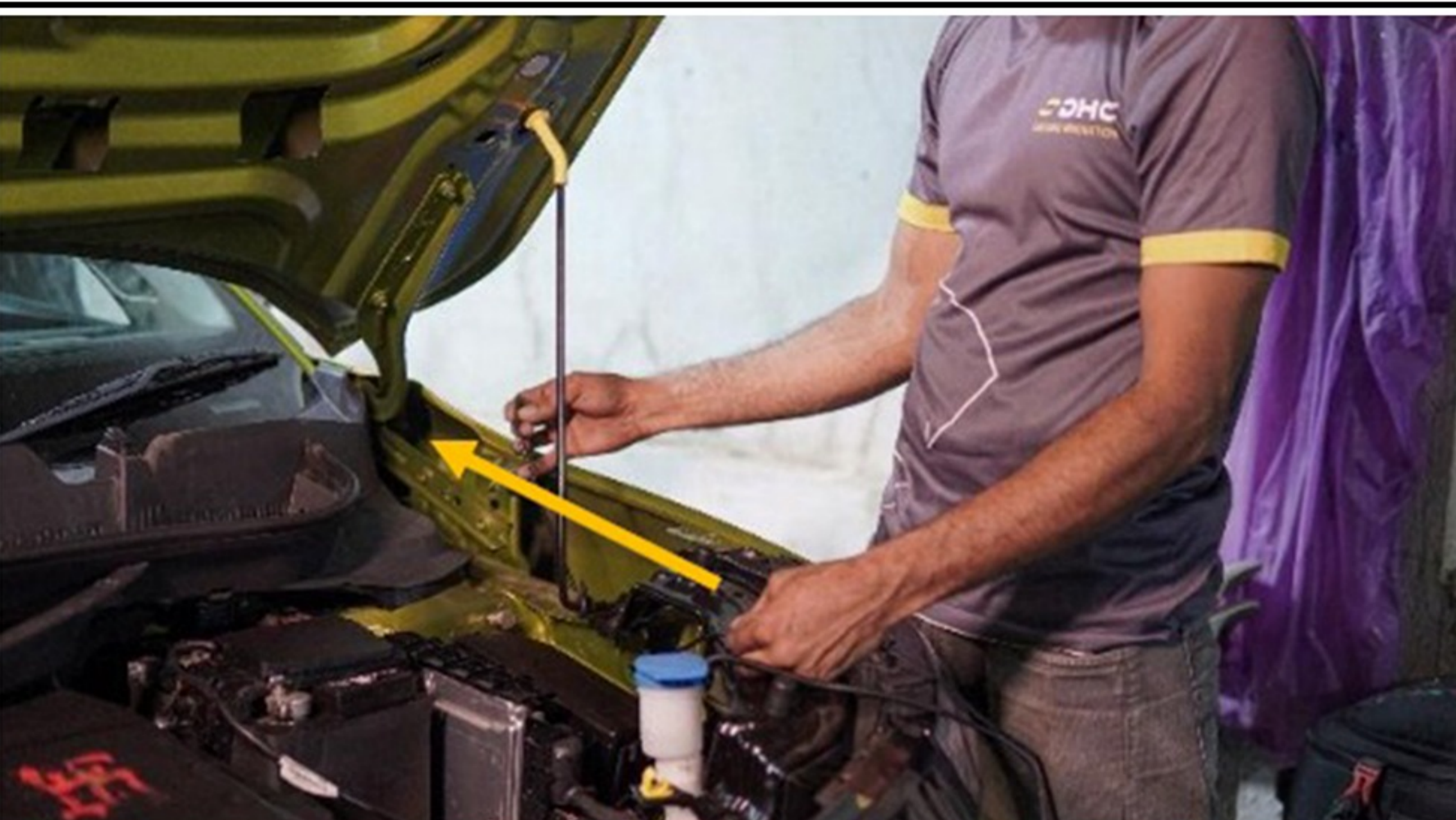
Step 88 :- Route Cable by fender edge till glove box (kindly refer the video if any confusion)
