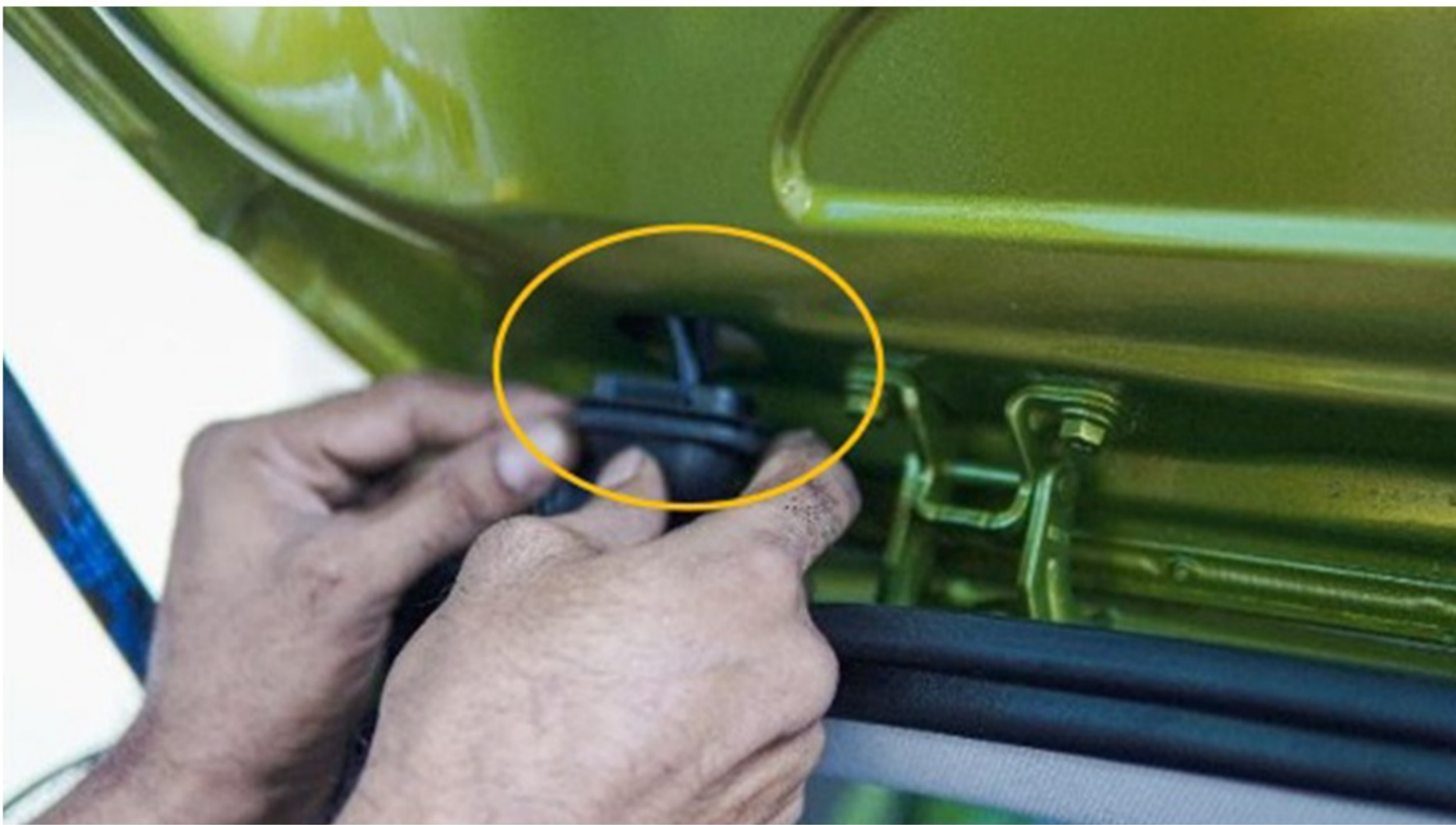
Step 67 :- Attach fitment top portion of rubber sleeve back as per series fitment
