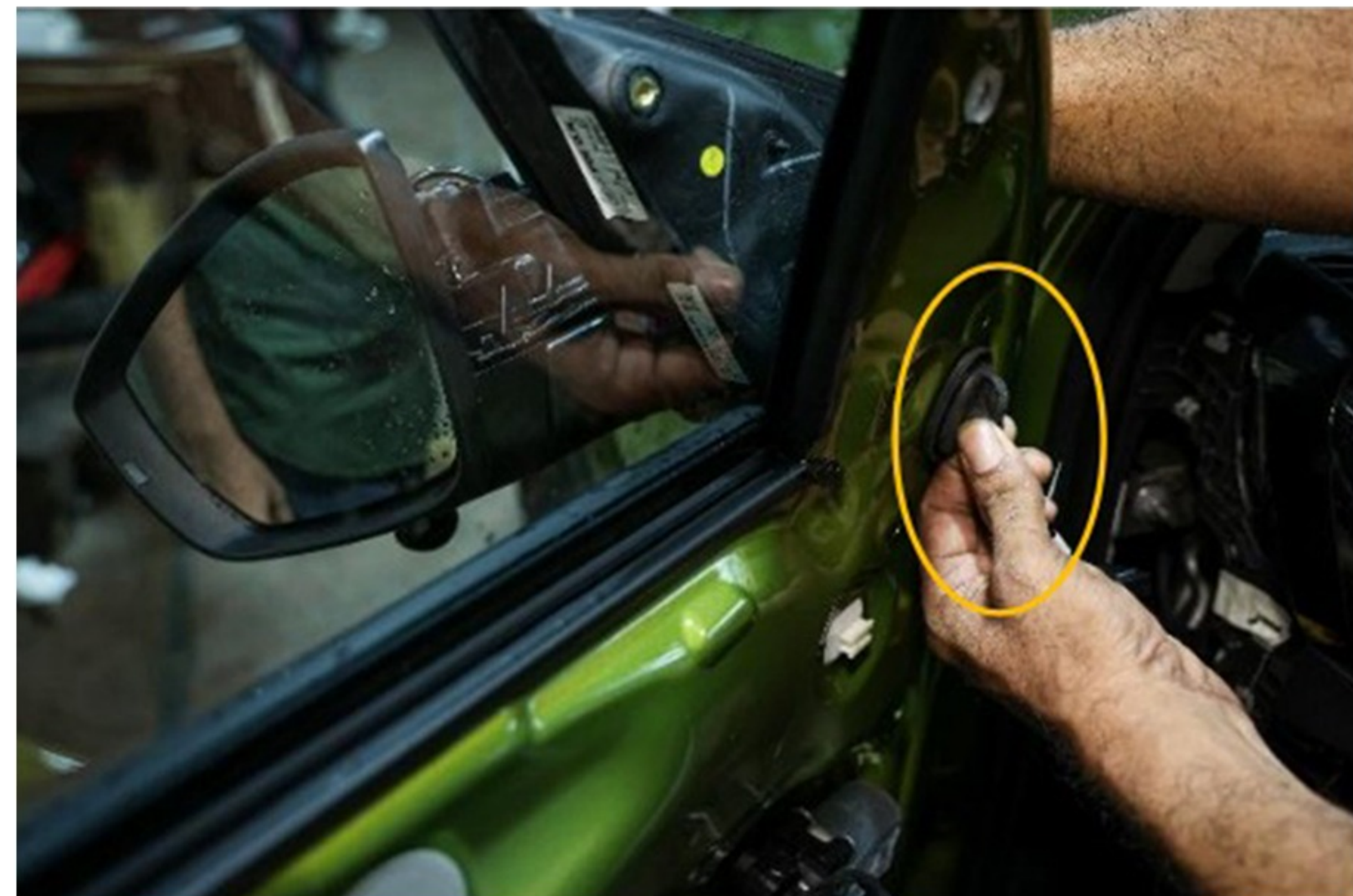
Step 40 :- Connect rubber caps properly
