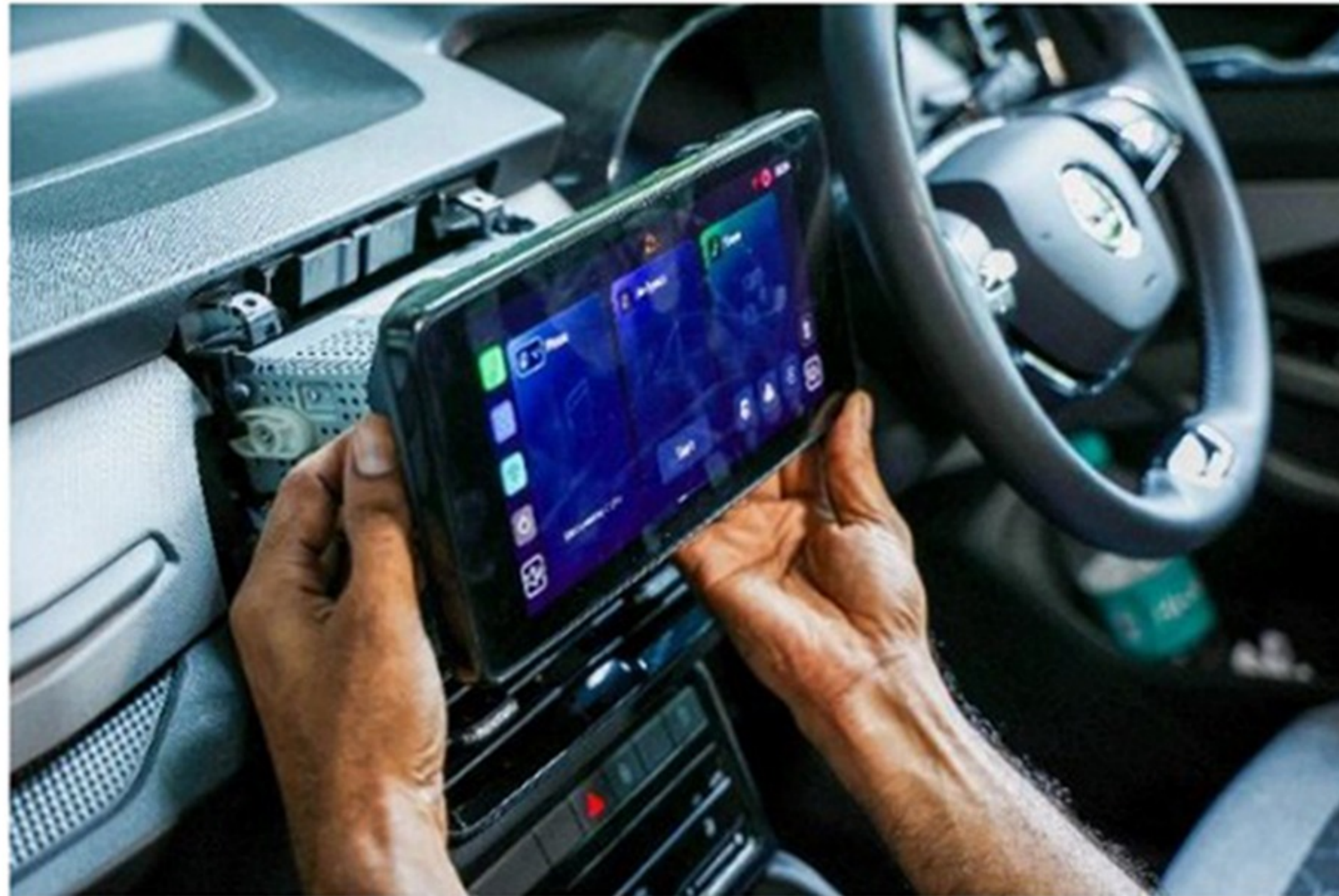
Step 3 :- Remove series Multimedia as per series disassembly
