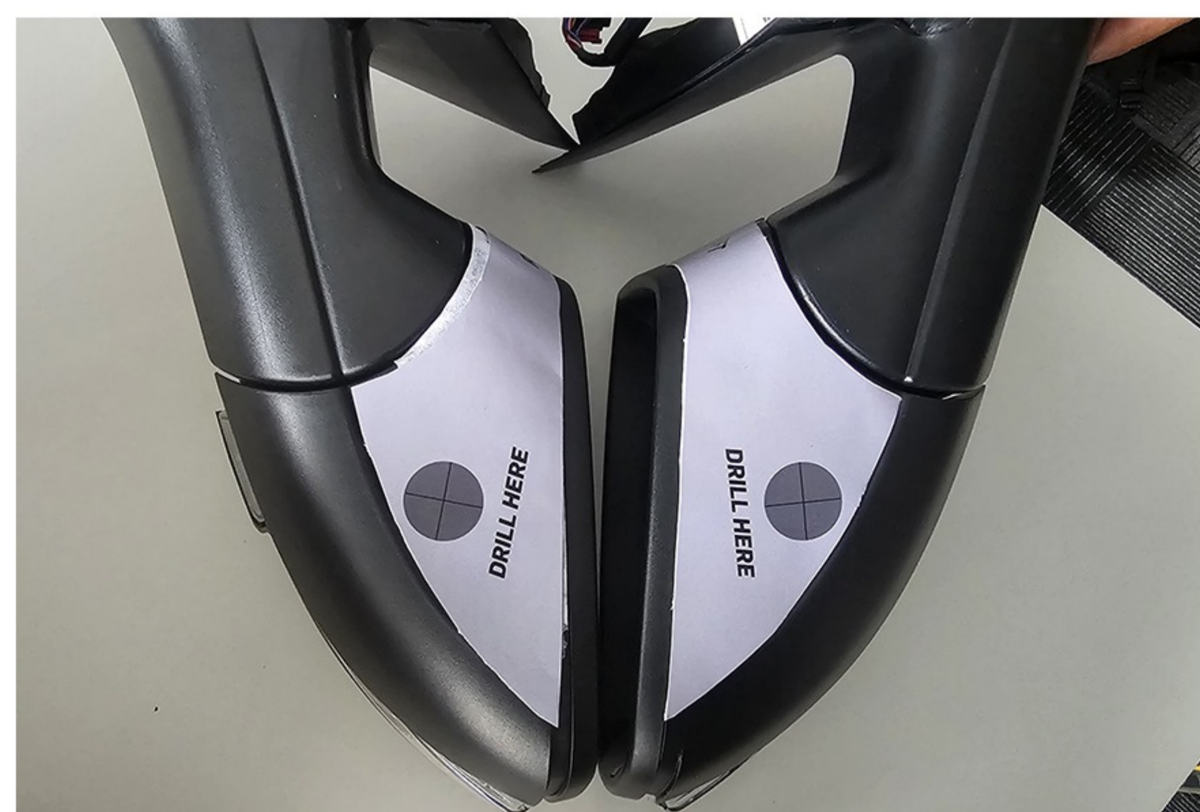
Step 32 :- Align ORVM Template as Shown PART 16
