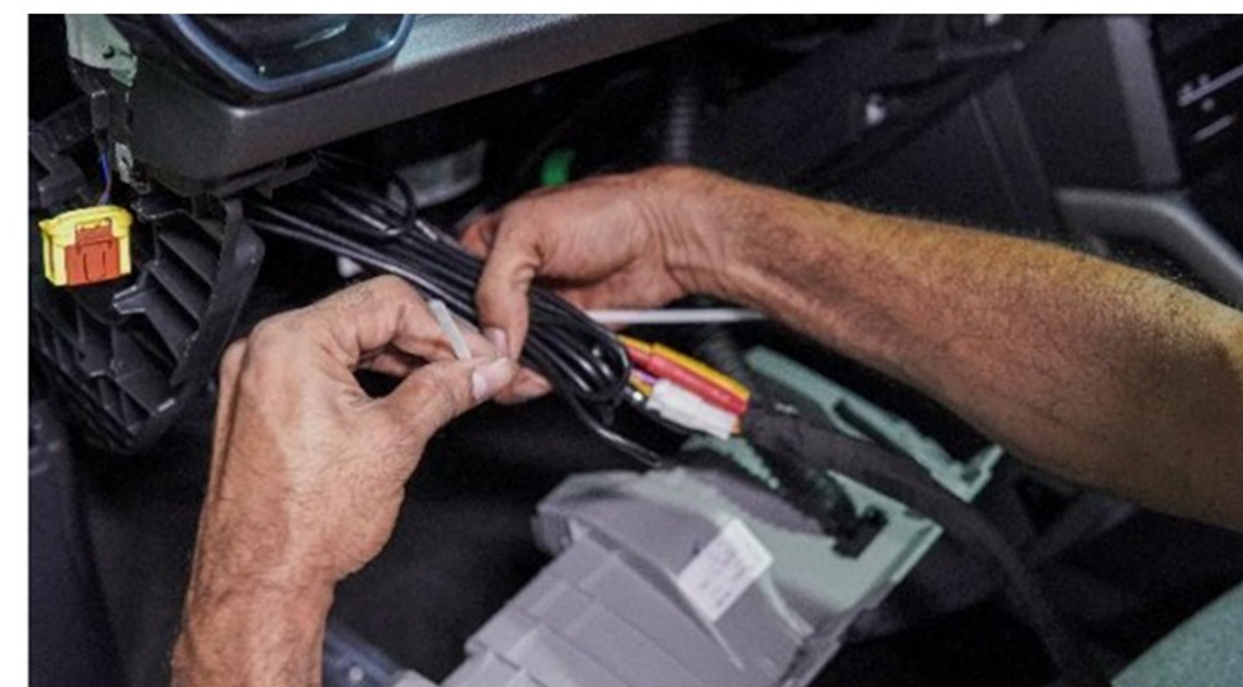
Step 105 :-Tie cable the (Part no 8) excess cables near the glove box
