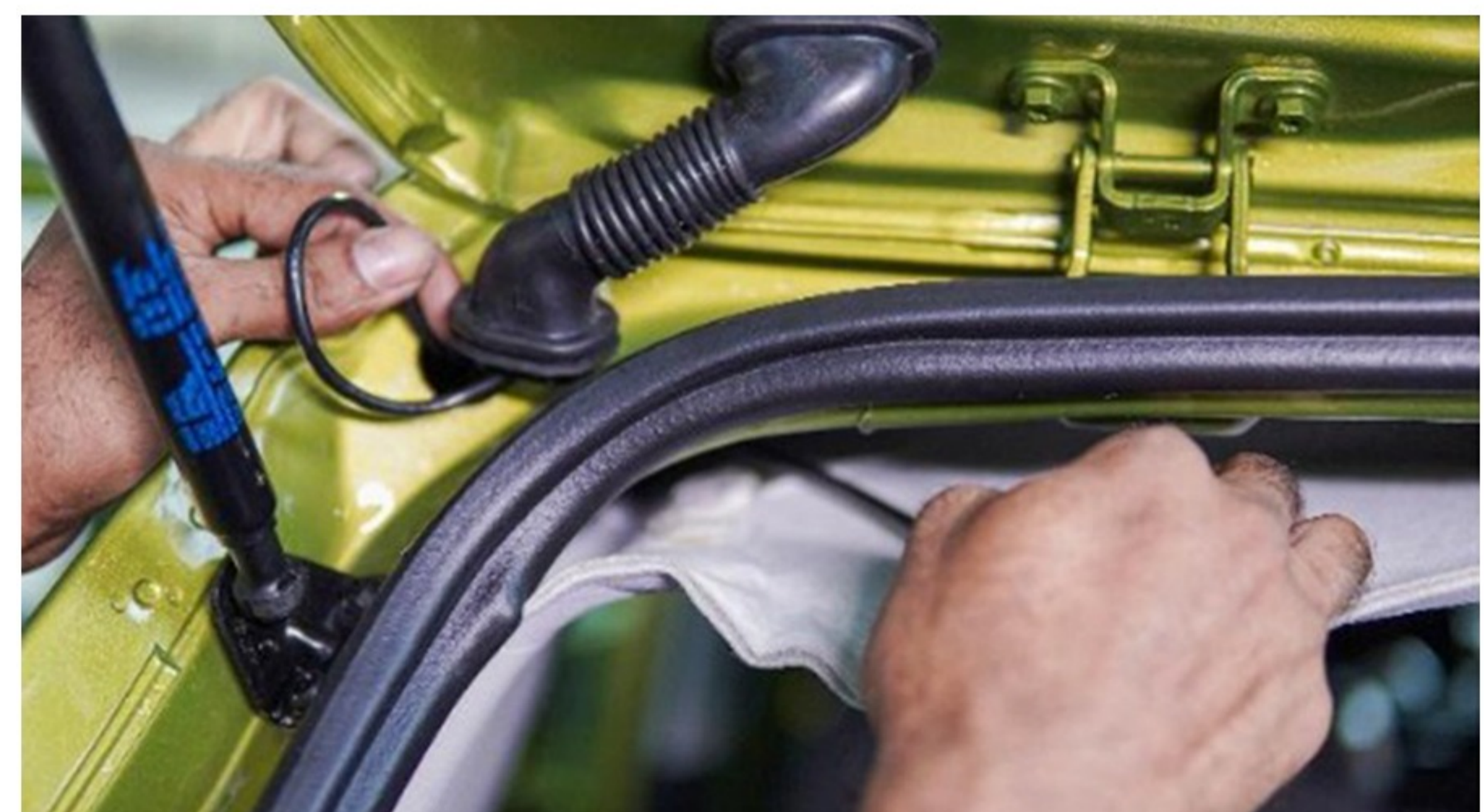
Step 70 :- Route the cable as shown from sleeve to roof liner.
