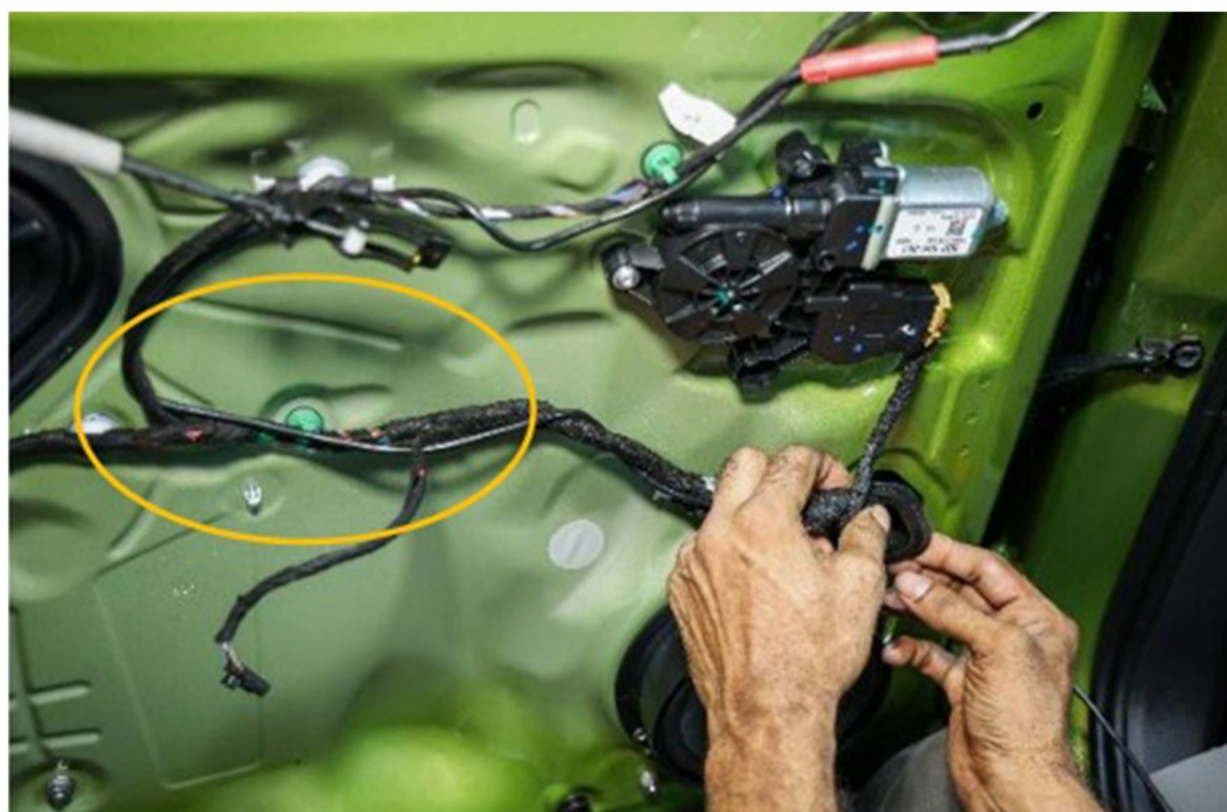
Step 45 :- route extension cable with the series cables
