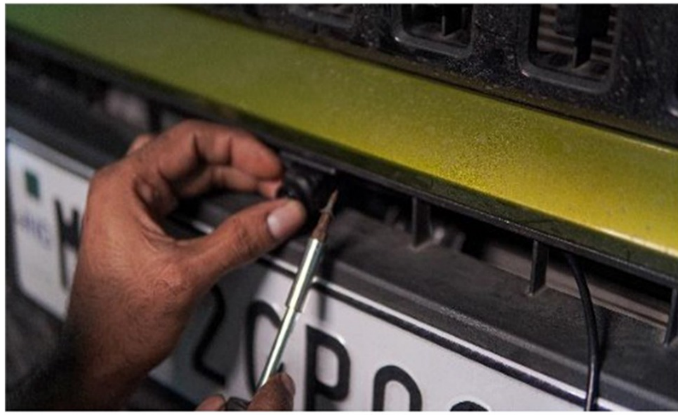
Step 82 :- Fit the camera with self tapping screw ( part no 12)
