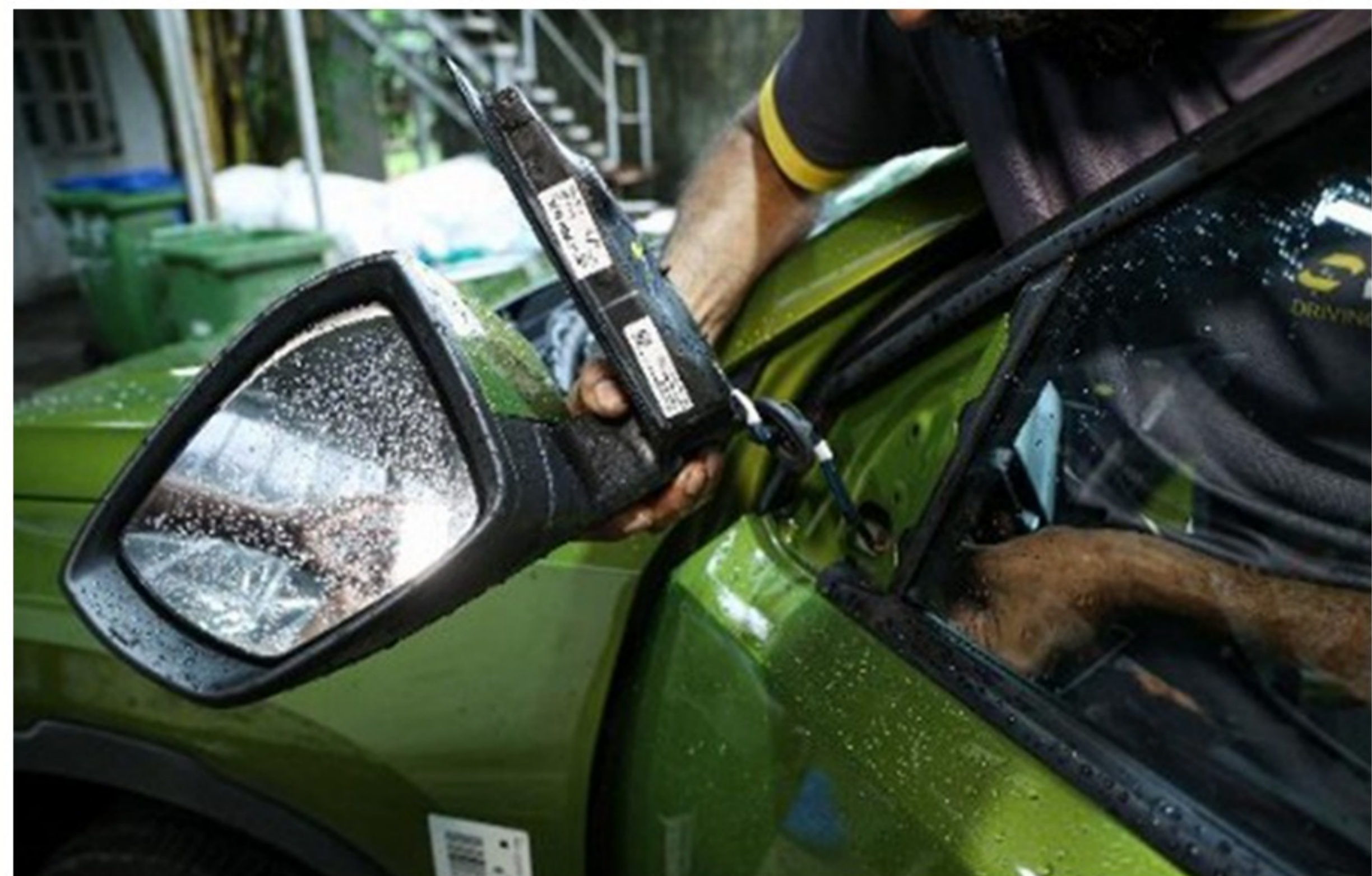
Step 30 :- Remove the Left and Right ORVM's carefully as per series
