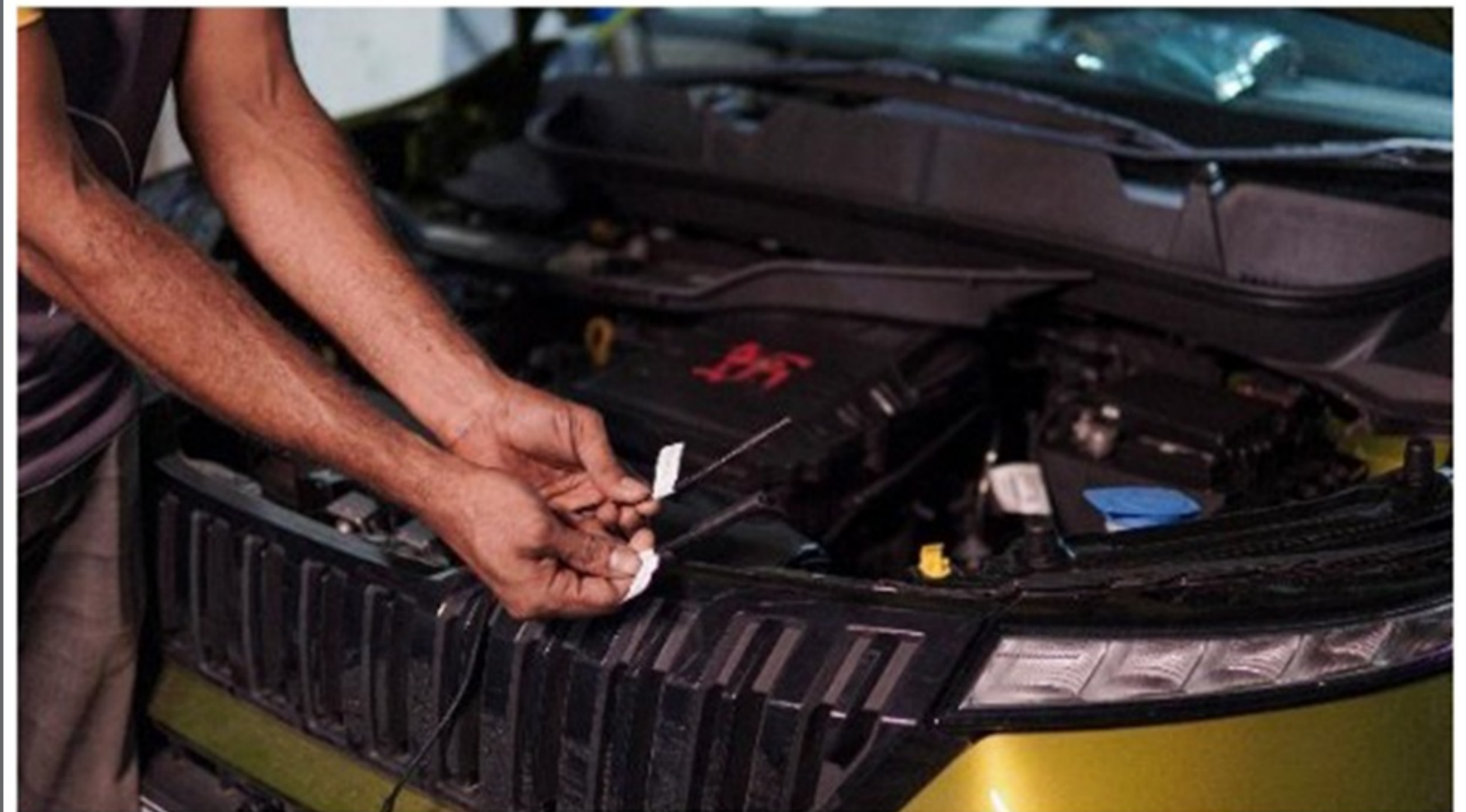
Step 85 :- Connect the Front Camera (Part no 7) and Front Extension Cable (Part no 5)
